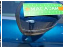
Outside rear-view mirror housing R, Scratch(es), Acceptable
