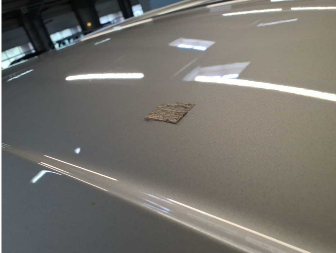
Damage 5: Roof: Roof - Glued / labelled - De-glue / neutralise
