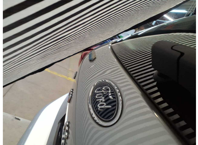
Damage 13: Boot lid / rear door: Boot lid - dent(s) - Smooth repair work
