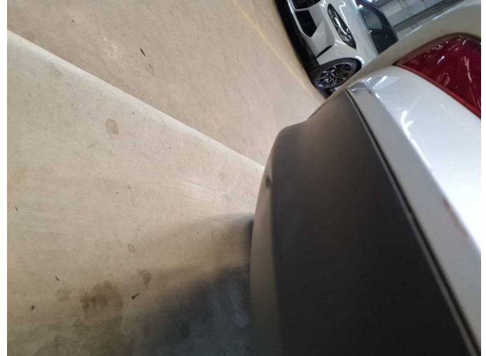
Damage 20: Rear bumper: Spoiler - Deformed - Replace
