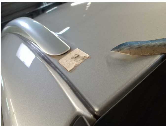
Damage 5: Roof: Roof - Glued / labelled - De-glu / neutralise
