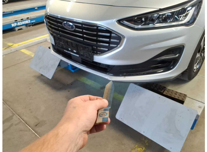
Damage 23: Front bumper: Front bumper - Deformed - Repair and paint
