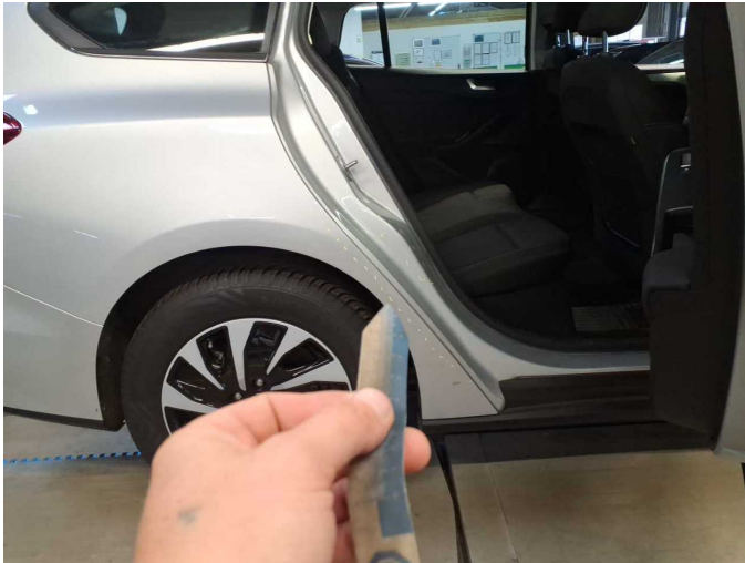
Damage 15: Side panel - rear right side: Side panel (+ Einstieg) - Scratch(es) - Smart repair
