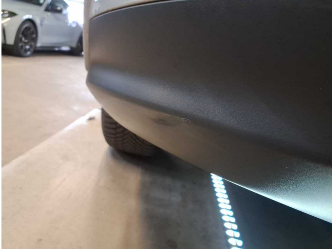
Damage 20: Rear bumper: Spoiler - Deformed - Replace
