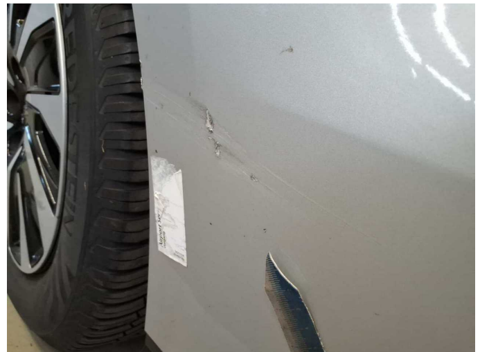
Damage 21: Rear bumper: Rear bumper - Scratched - Repair and paint
