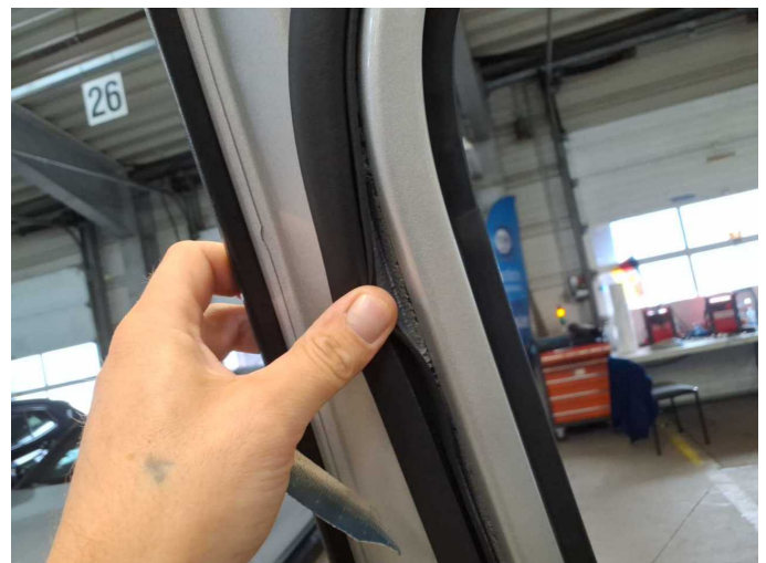
Damage 3: Door - front left side: Door seal - Loose - Repair
