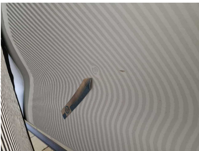
Damage 22: Door - front left side: Door - Dent / paintcoat damage - Repair and paint
