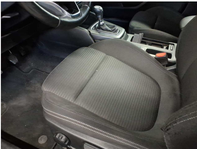
Damage 12: Seat - front: Seat cover - left side - Burn hole (cigarettes) - Smart repair
