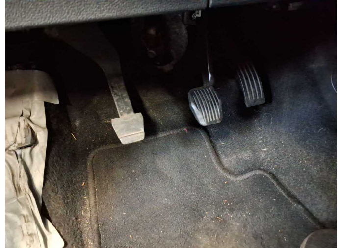
Damage 1: Pedal system: Clutch pedal cover / rubber - Missing - Replace
