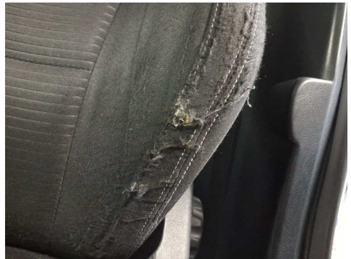
Damage 17: Seat - front: Seat cover - left side (Wange) - Broken / torn - Replace
