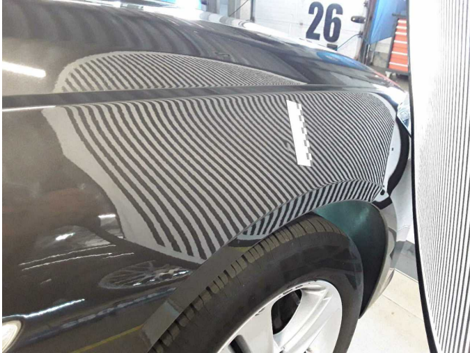
Damage 11: Mudguard - right side: Mudguard - right side - dent(s) - Smooth repair work
