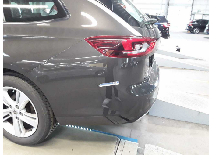
Damage 18: Rear bumper: Rear bumper - Scratch(es) - Paint
