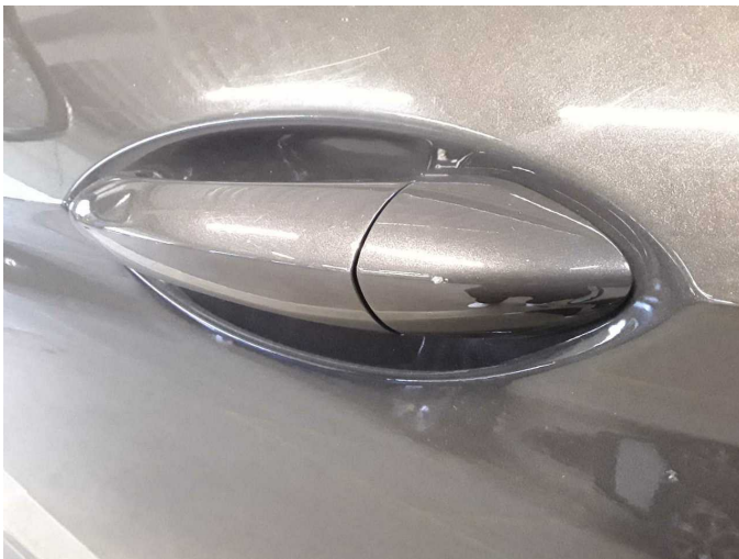
Damage 6: Door - front left side: Door handle - outside - Scratch(es) - Smart repair
