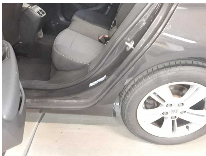
Damage 17: Body: C-pillar - left side - Dent / paintcoat damage - Repair and paint
