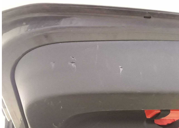
Damage 15: Boot lid / rear door: Trim - standard - lower - Scratched - Loss in value
