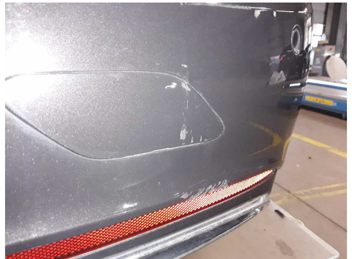
Damage 18: Rear bumper: Rear bumper - Scratch(es) - Paint
