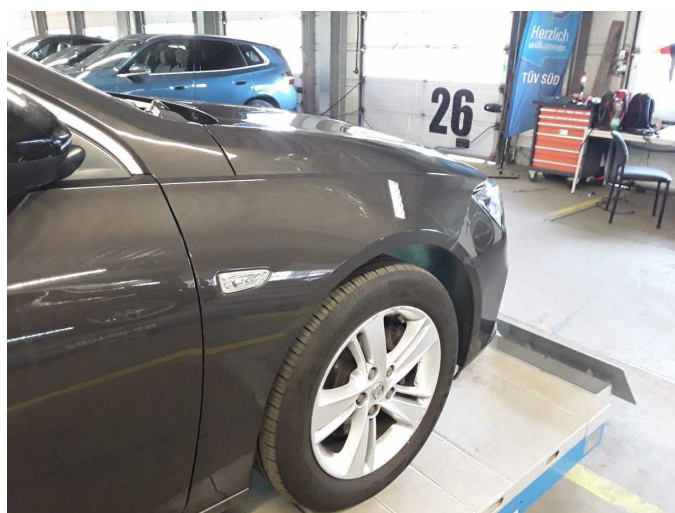
Damage 11: Mudguard - right side: Mudguard - right side - dent(s) - Smooth repair work
