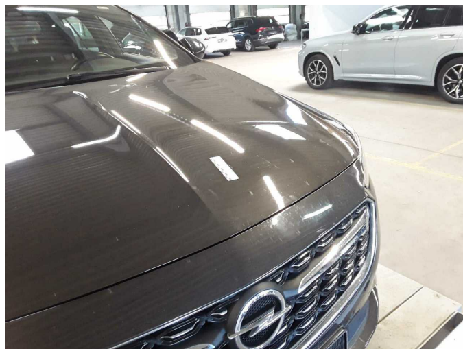
Damage 9: Bonnet: Bonnet - dent(s) - Smooth repair work
