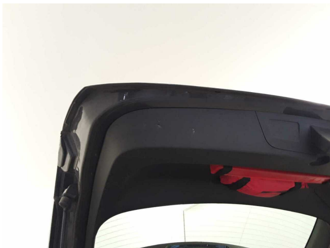
Damage 15: Boot lid / rear door: Trim - standard - lower - Scratched - Loss in value
