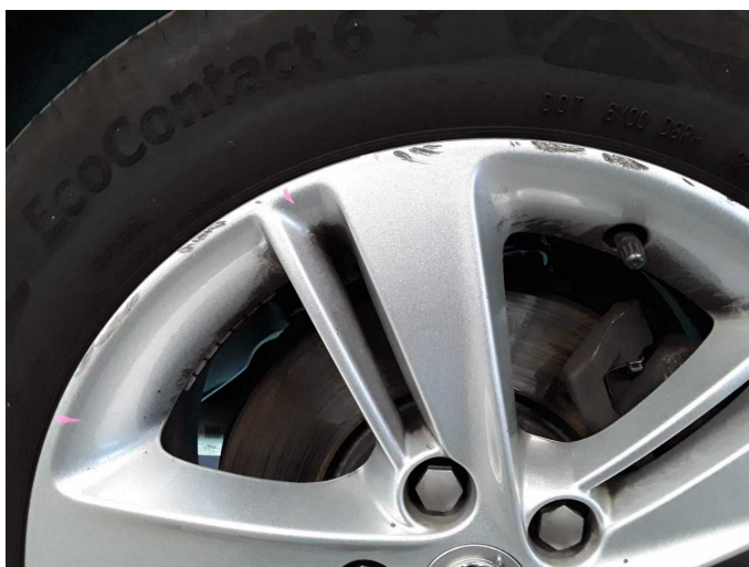
Damage 16: Wheel / tyres: Alloy rim - front right side (Materialabtrag) - Scratch(es) - Replace
