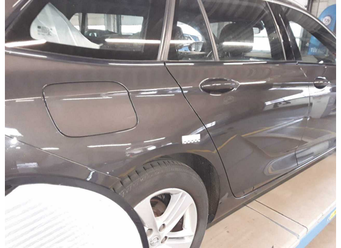
Damage 12: Side panel - rear right side: Side panel - dent(s) - Smooth repair work
