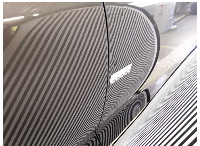
Damage 13: Door - front right side: Door - dent(s) - Smooth repair work
