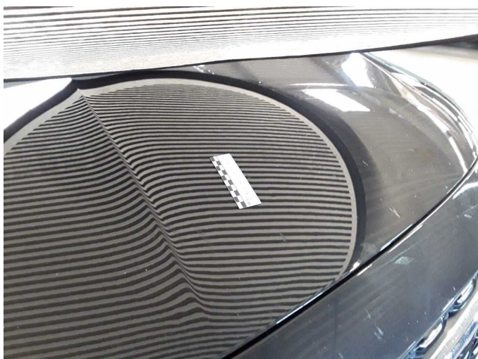
Damage 9: Bonnet: Bonnet - dent(s) - Smooth repair work
