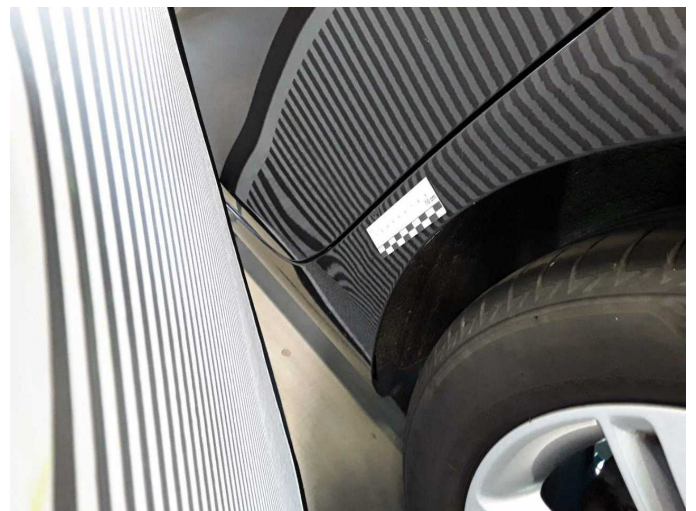
Damage 14: Side panel - rear left side: Side panel - dent(s) - Smooth repair work
