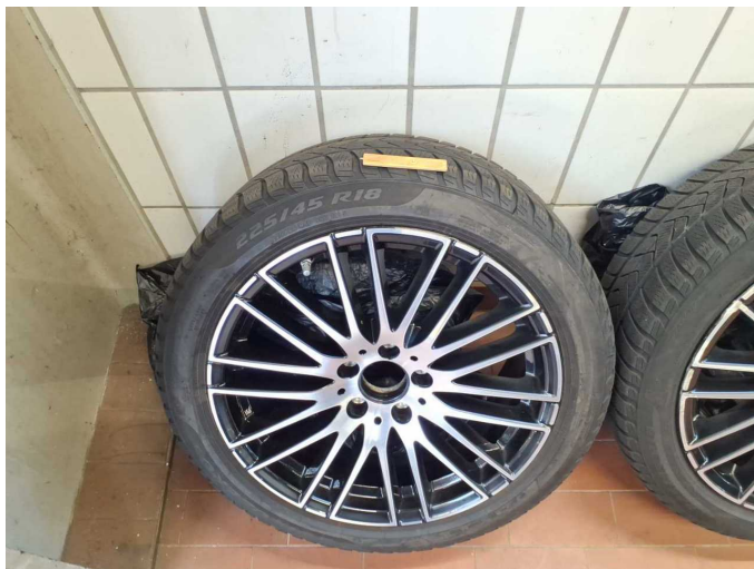
Damage 10: 2nd wheel set: 2 tyres (4mm) - Does not meet the leasing specifications - Replace
