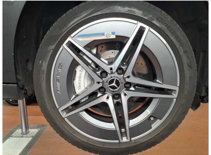
Damage 14: Wheel / tyres: Alloy rim - front right side - Scratched - Loss in value
