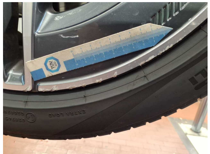
Damage 13: Wheel / tyres: Alloy rim - front left side - Scratched - Loss in value
