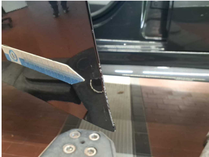
Damage 9: Door - front left side: Door edge - Dent / paintcoat damage - Smart repair
