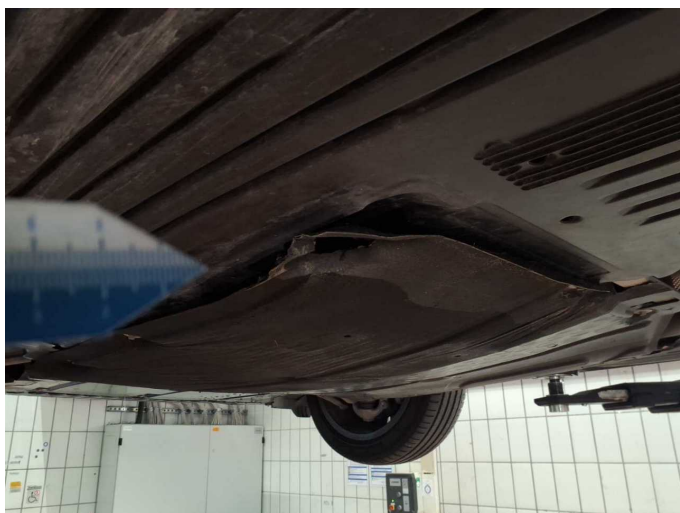
Damage 8: Body: Underbody panelling - Broken / torn - Replace
