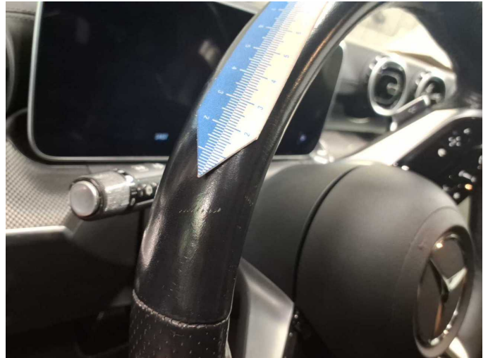
Wear and tear 4: Steering system: Steering wheel - Scratch(es) - No deduction
