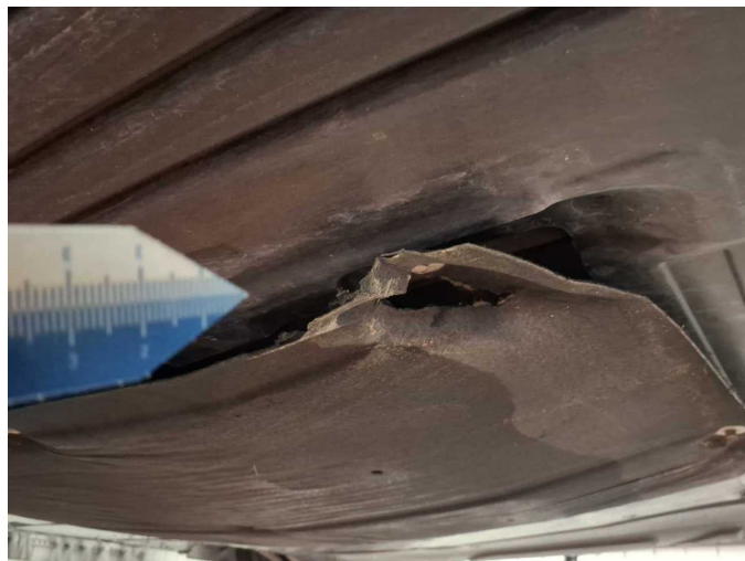
Damage 8: Body: Underbody panelling - Broken / torn - Replace
