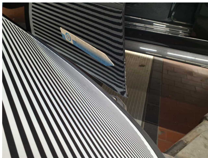
Damage 9: Door - front left side: Door edge - Dent / paintcoat damage - Smart repair
