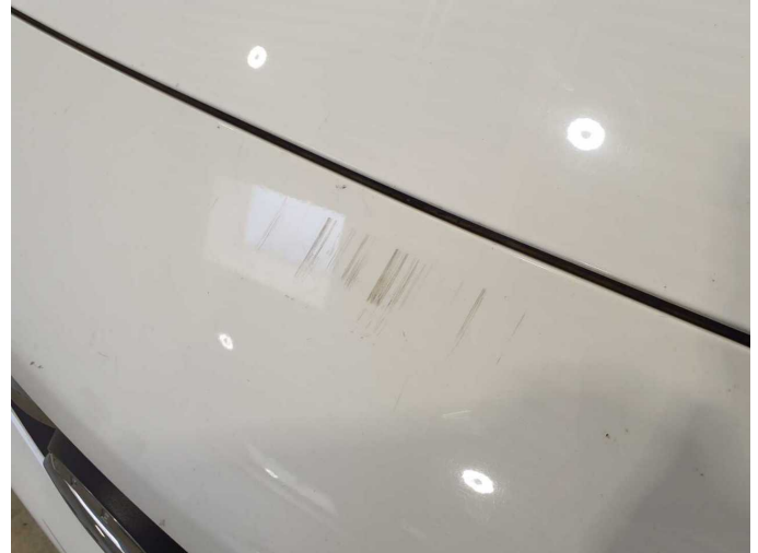
Damage 14: Front bumper: Front bumper - Scratch(es) - Paint
