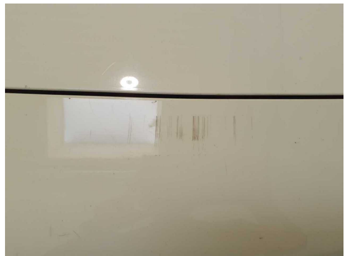
Damage 14: Front bumper: Front bumper - Scratch(es) - Paint
