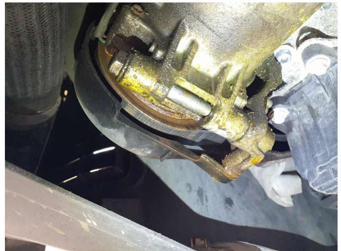
Damage 5: Engine: Engine - Leaking - Perform diagnosis
