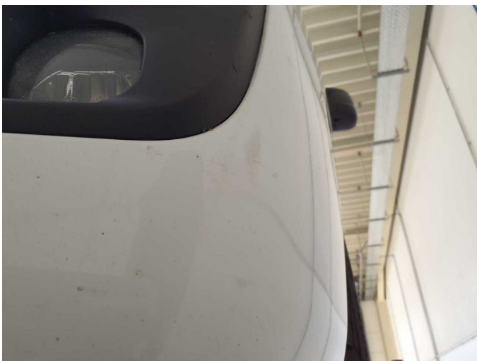
Damage 14: Front bumper: Front bumper - Scratch(es) - Paint
