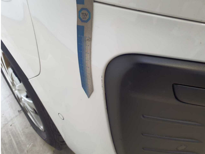
Damage 14: Front bumper: Front bumper - Scratch(es) - Paint
