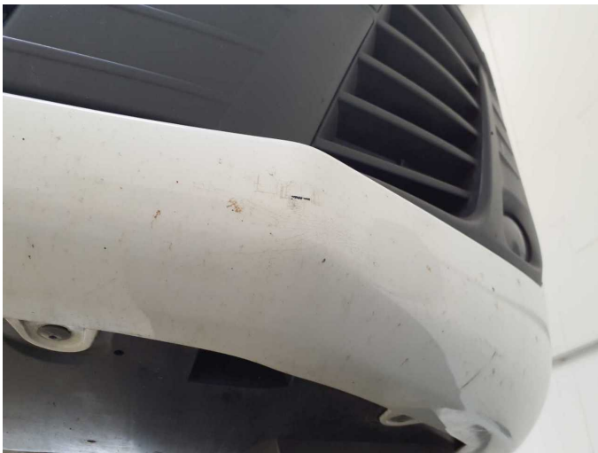
Damage 14: Front bumper: Front bumper - Scratch(es) - Paint
