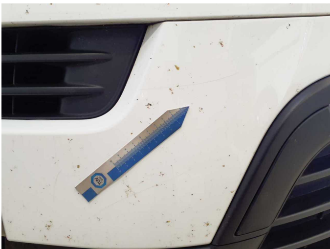
Damage 14: Front bumper: Front bumper - Scratch(es) - Paint
