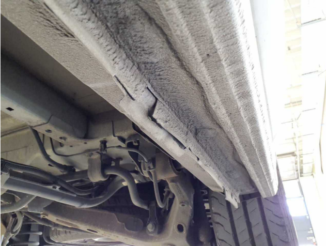
Damage 9: Sill - left side: Sill - dent(s) - Repair and paint
