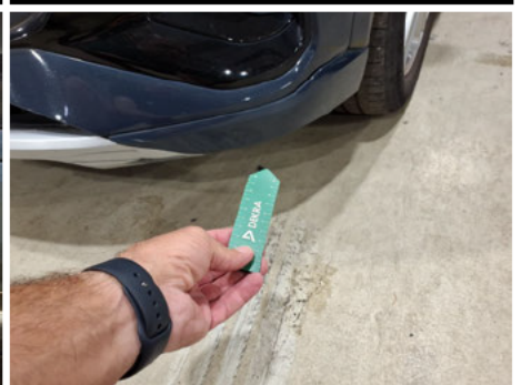
Bumper moulding / Front Left / Scratched
