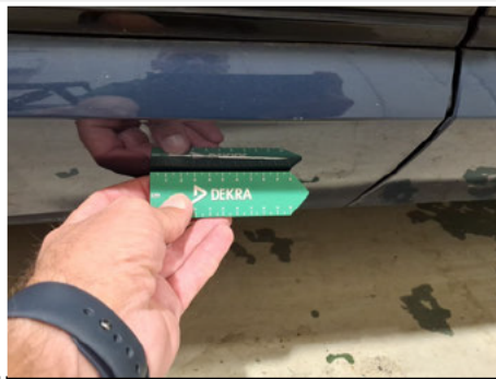
Door moulding / Back Right / Scratched
