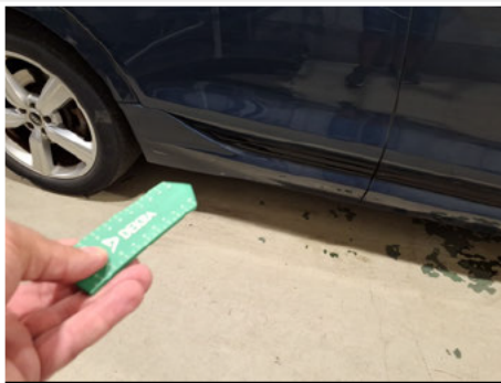
Door moulding / Back Right / Scratched
