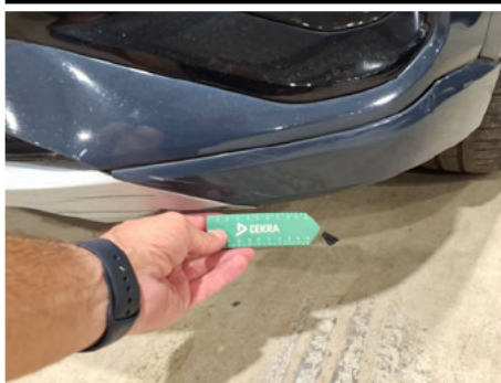
Bumper moulding / Front Left / Scratched
