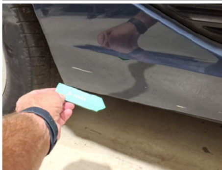
Door moulding / Back Right / Scratched
