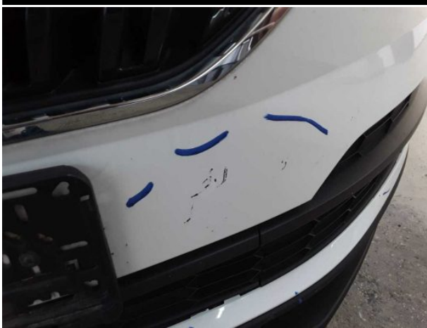
Damage #23: Front bumper: Front bumper - Damaged - Replace
