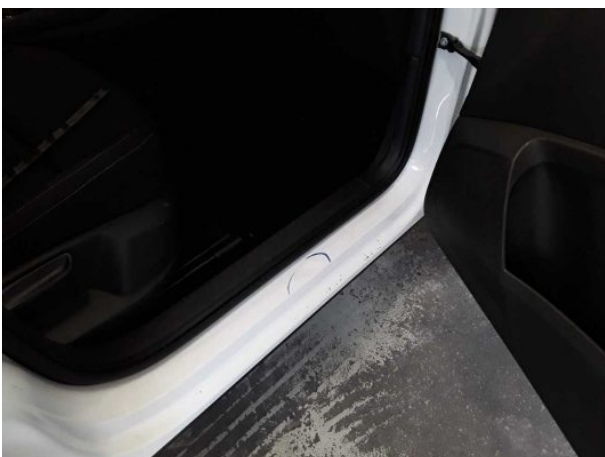
Damage #9: Sill - right side: Sill - dent(s) - Smooth repair work
