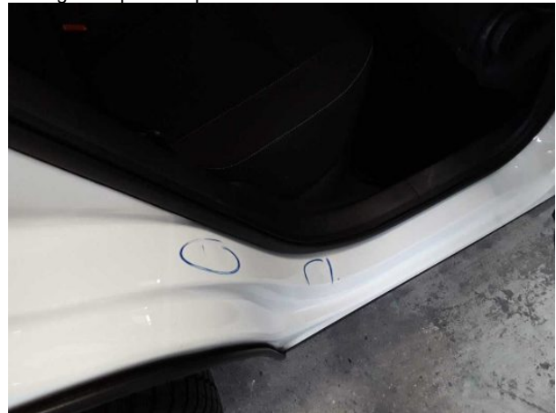
Damage #21: Side panel - rear right side: Sill - Dent / paintcoat damage - Repair and paint
