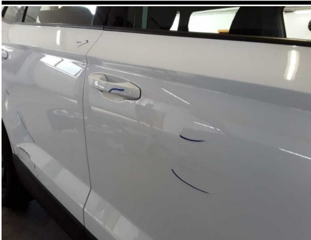
Damage #22: Door - front right side: Door - Dent / paintcoat damage - Repair and paint
