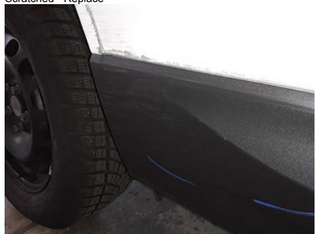
Damage #16: Door - rear right side: Brightware - lower - Scratched - Replace
