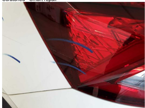
Damage #13: Tail light: Tail lamp - left side - Scratched - Replace
