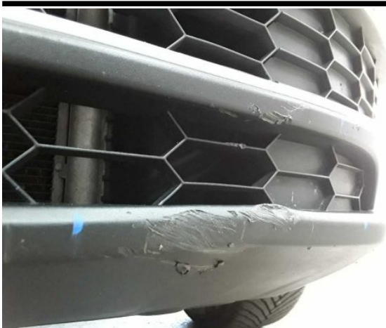
Damage #19: Front bumper: Spoiler - Scratched - Replace
