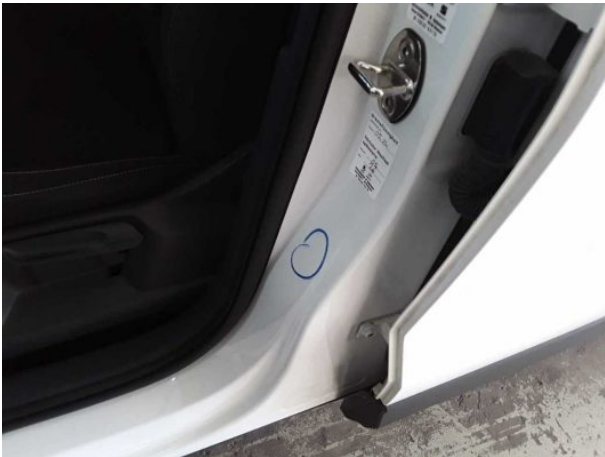
Damage #8: Sill - left side: Sill - dent(s) - Smooth repair work
