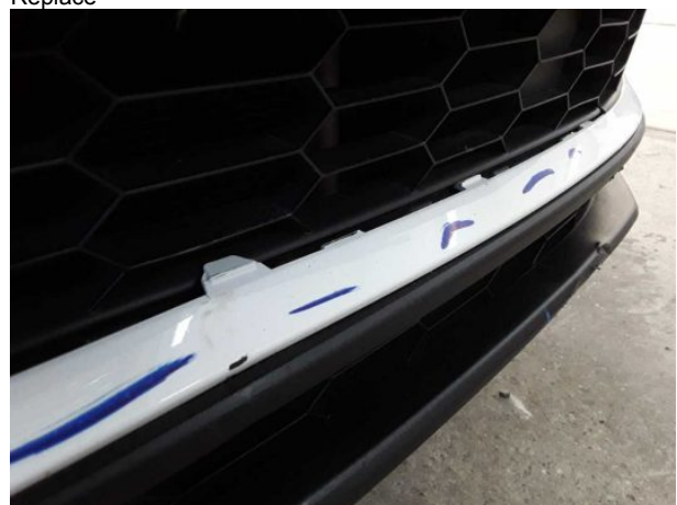
Damage #23: Front bumper: Front bumper - Damaged - Replace
