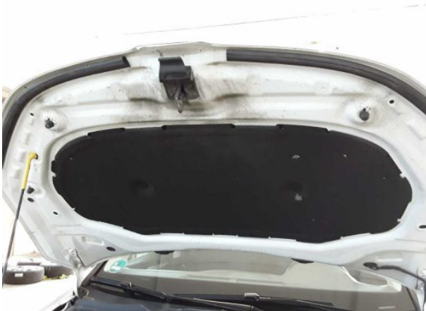
Damage #6: Bonnet: Insulation lining - Damage caused by marte... rodent - Replace
