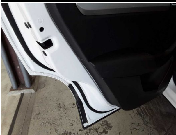
Damage #17: Door - rear left side: Door - dent(s) - Smooth repair work
