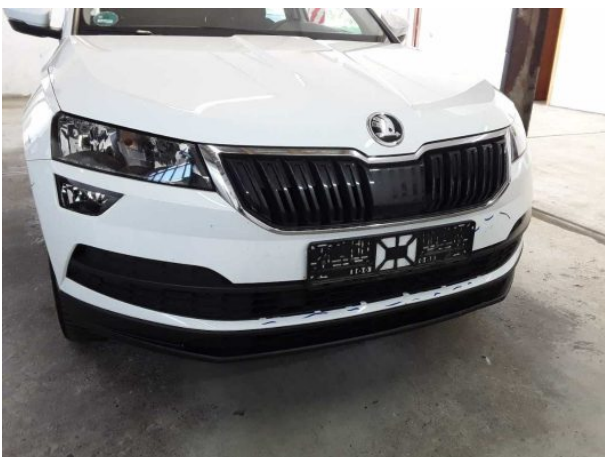
Damage #19: Front bumper: Spoiler - Scratched - Replace
