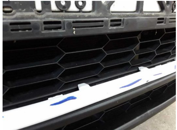
Damage #18: Front bumper: Grille - Deformed - Replace
