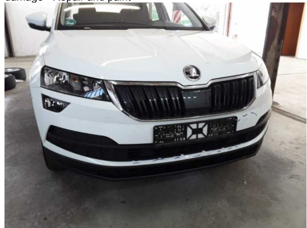
Damage #23: Front bumper: Front bumper - Damaged - Replace
