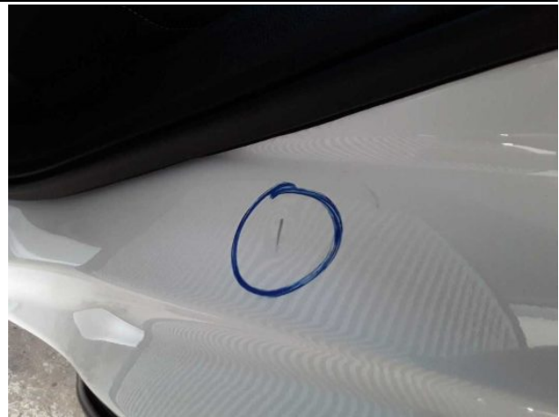
Damage #20: Side panel - rear left side: Sill - Dent / paintcoat damage - Repair and paint
