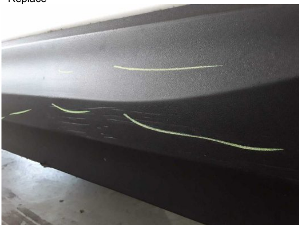
Damage #15: Door - front right side: Brightware - lower - Scratched - Replace
