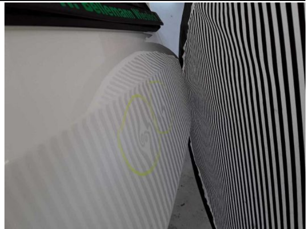
Damage #14: Boot lid / rear door: Boot lid - dent(s) - Smooth repair work
