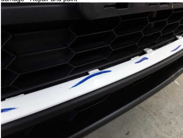
Damage #23: Front bumper: Front bumper - Damaged - Replace
