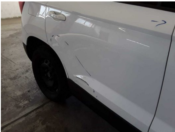
Damage #24: Door - rear right side: Door - Deformed - Replace
