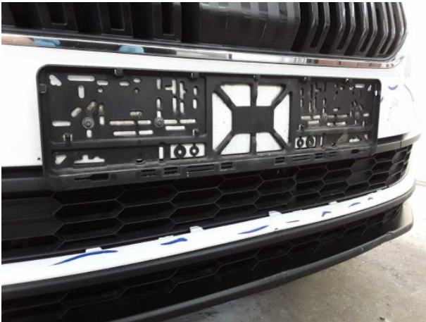
Damage #18: Front bumper: Grille - Deformed - Replace
