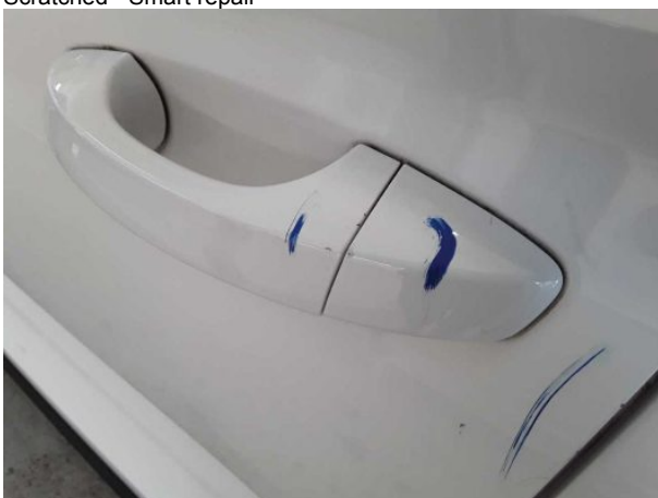
Damage #12: Door - front left side: Door handle - outside - Scratched - Smart repair
