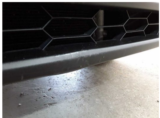
Damage #19: Front bumper: Spoiler - Scratched - Replace
