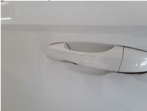
Damage #11: Door - rear left side: Door handle - outside - Scratched - Smart repair
