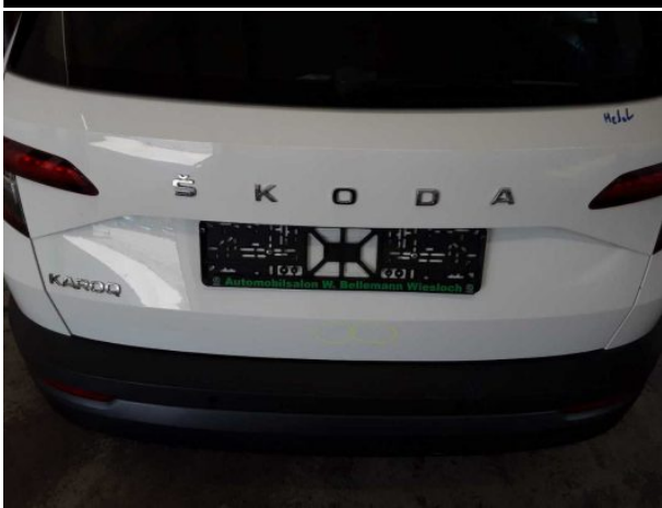
Damage #14: Boot lid / rear door: Boot lid - dent(s) - Smooth repair work
