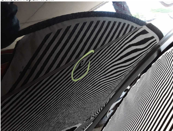
Damage #4: Door - rear left side: Door - Dent / paintcoat damage - Smooth repair work
