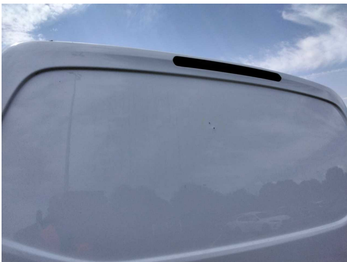
Damage 3: Boot lid / rear door: Boot lid - Dent / paintcoat damage - Smart repair
