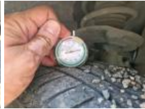
Tyre FL, Out of tolerance, Replace
