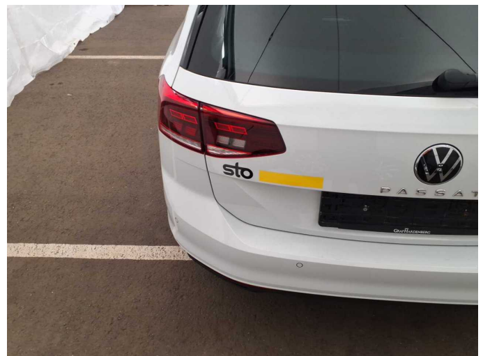
Damage 1: Body: Body - Glued / labelled - De-glug / neutralise
