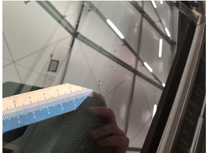
Damage 4: Vehicle glazing: Windscreen - Broken / torn - repair according to calculation
