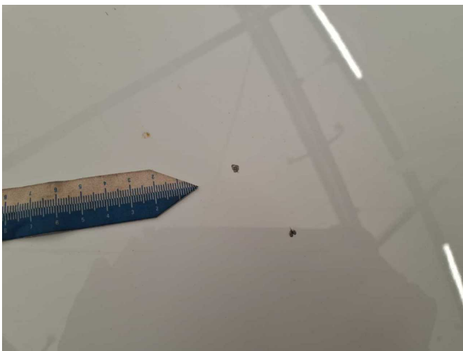
Damage 3: Bonnet: Bonnet - Stone chips - Paint
