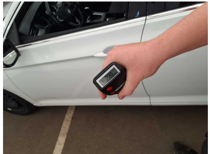
Repainting 3: Door - front left side
