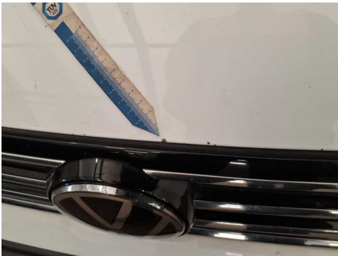
Damage 3: Bonnet: Bonnet - Stone chips - Paint
