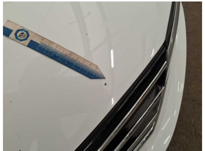
Damage 3: Bonnet: Bonnet - Stone chips - Paint
