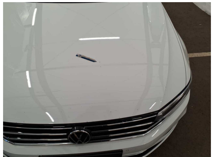
Damage 3: Bonnet: Bonnet - Stone chips - Paint
