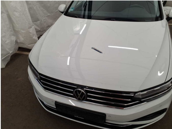
Damage 3: Bonnet: Bonnet - Stone chips - Paint
