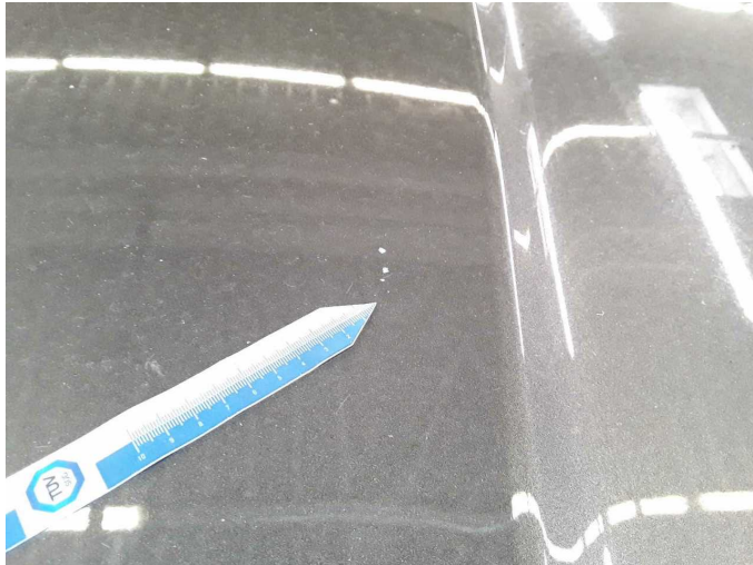
Damage 2: Bonnet: Bonnet - Stone chips - Paint
