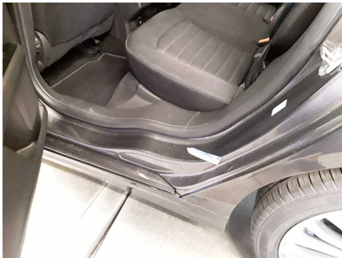
Wear and tear 1: Side panel - rear left side: Sill - Scratched - No deduction
