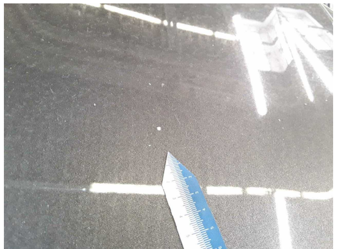
Damage 2: Bonnet: Bonnet - Stone chips - Paint
