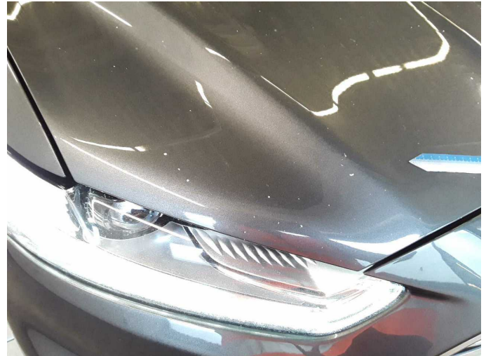
Damage 2: Bonnet: Bonnet - Stone chips - Paint
