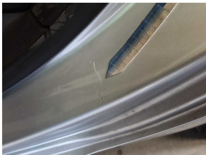
Damage 6: Side panel - rear left side: Elbow - Scratched - Smart repair
