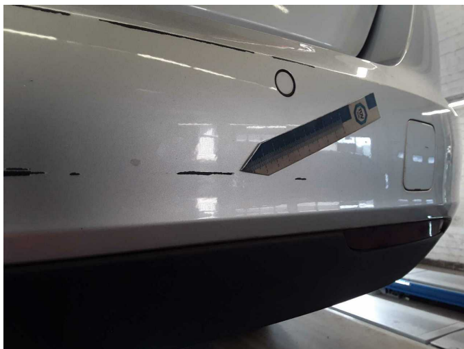
Damage 10: Rear bumper: Rear bumper - Scratched - Repair and paint
