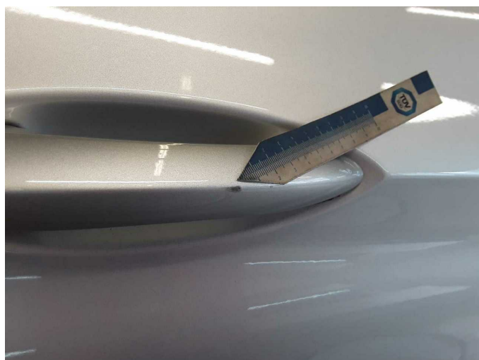
Damage 5: Door - front right side: Door handle - outside - Scratch(es) - Paint
