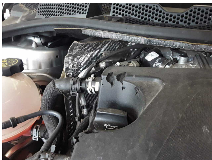
Damage 8: Engine: Engine cover - Broken / torn - Replace
