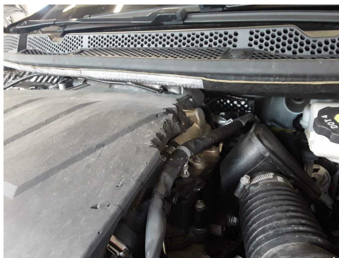
Damage 8: Engine: Engine cover - Broken / torn - Replace
