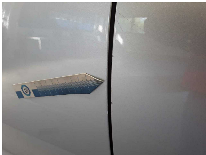
Damage 7: Door - front left side: Door edge - Scratched - Smart repair
