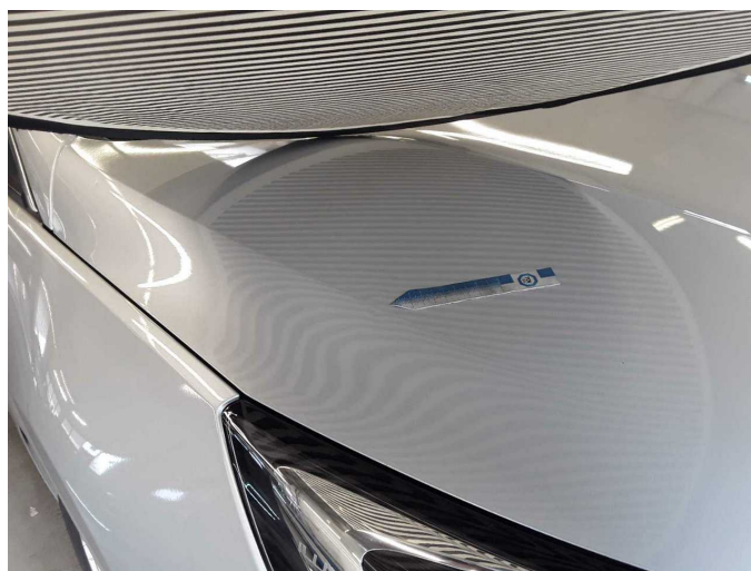
Damage 12: Bonnet: Bonnet - Dent / paintcoat damage - Repair and paint
