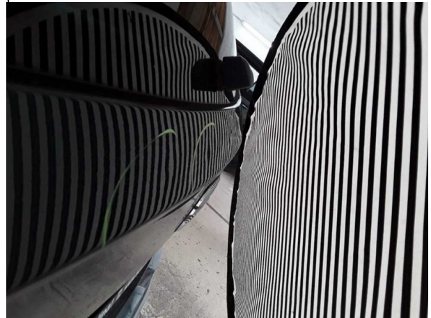
Damage #9: Boot lid / rear door: Boot lid - dent(s) - Repair and paint
