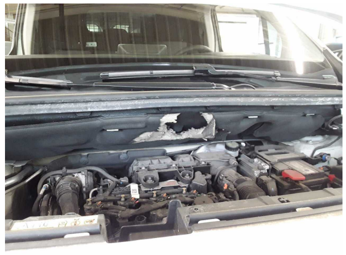
Damage 2: Cab: Insulation lining - Damaged - Replace
