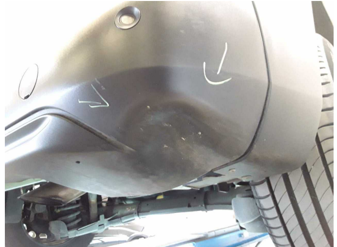
Damage 3: Rear bumper: Rear bumper (unpainted) - Deformed - Replace
