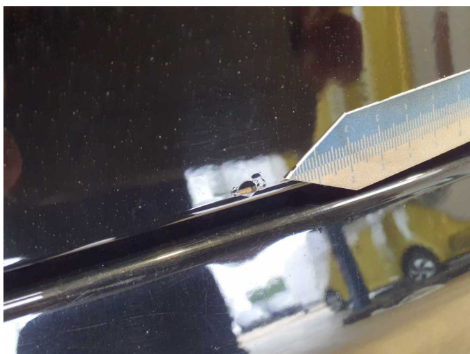
Damage 4: Boot lid / rear door: Boot lid - Corrosion - Repair and paint
