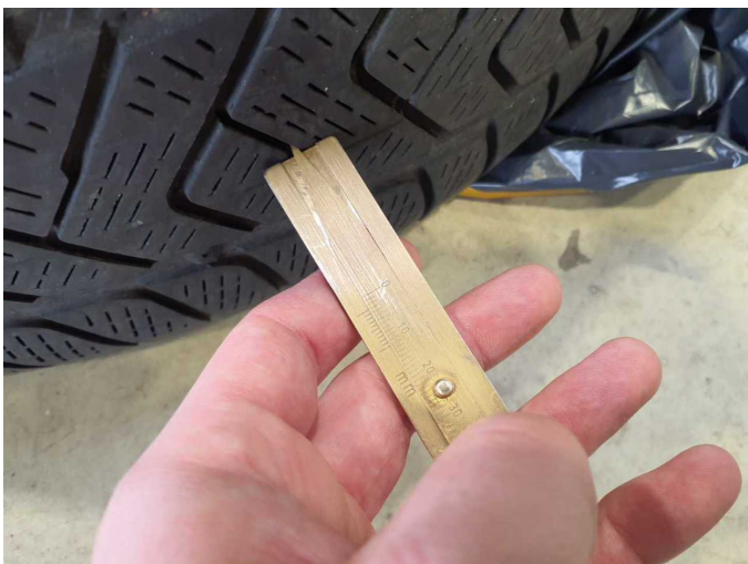
Damage 3: 2nd wheel set: 2 tyres - Does not meet the leasing specifications - Replace
