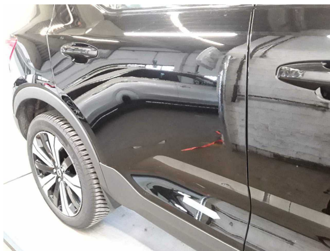
Damage 4: Door - rear right side: Door - Deformed - Repair and paint
