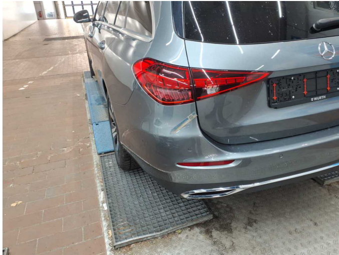
Damage 7: Rear bumper: Rear bumper - Scratch(es) - Paint
