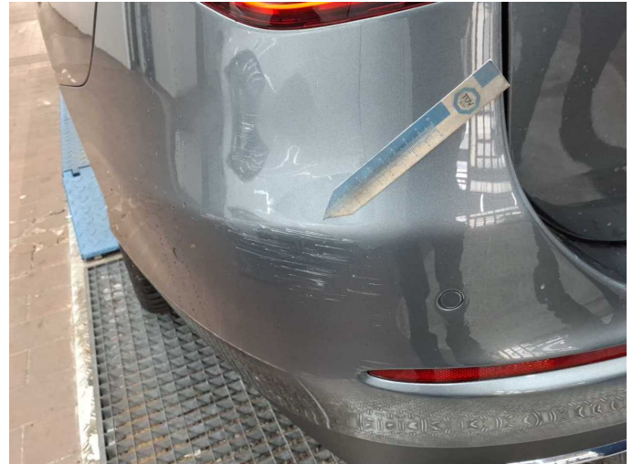
Damage 7: Rear bumper: Rear bumper - Scratch(es) - Paint
