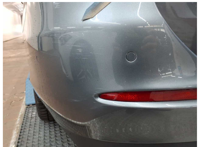
Damage 7: Rear bumper: Rear bumper - Scratch(es) - Paint
