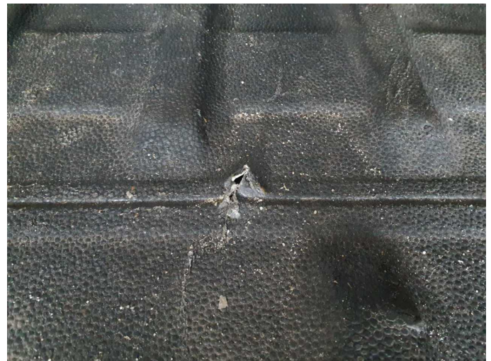
Damage 3: Trim / covers: Floor covering - rear right side (Laderaum) - Damaged - Replace
