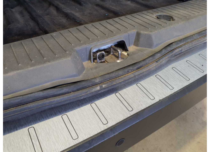
Damage 2: Boot lid / rear door: Seal - Deformed - Replace
