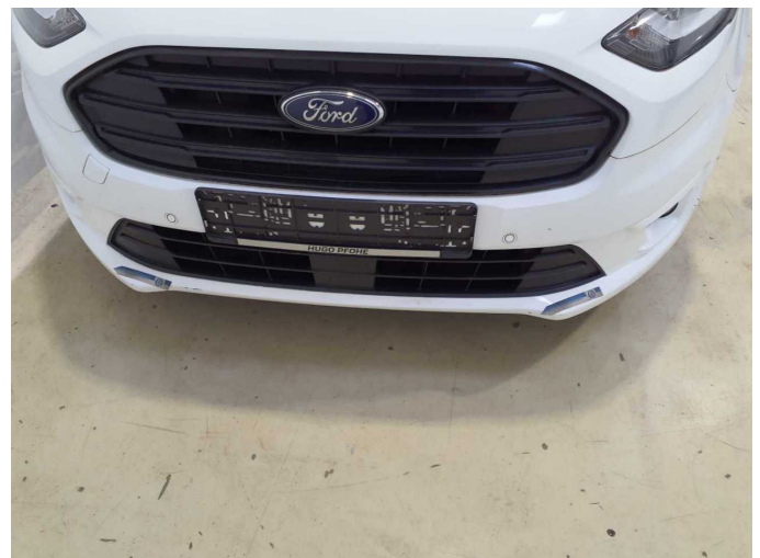
Damage 4: Front bumper: Front bumper - Dent / paintcoat damage - Repair and paint
