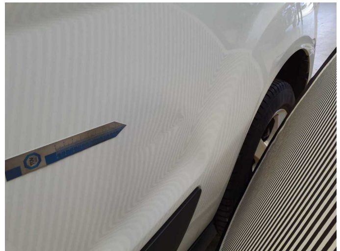
Damage 5: Side panel - rear left side: Side panel (Unterhalb) - dent(s) - Repair and paint
