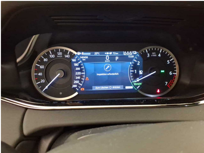
Damage 3: Misc.: Inspection / maintenance - Due - Perform
