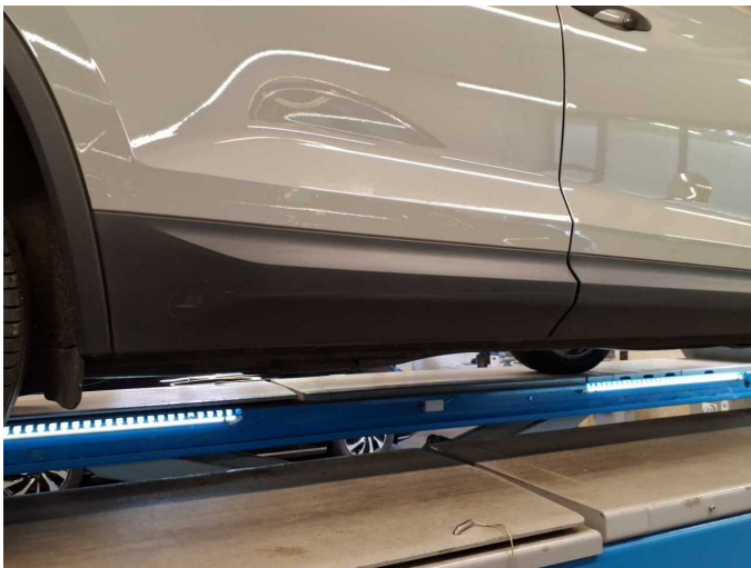
Damage 2: Door - rear right side: Brightware - lower - Scratch(es) - Replace
