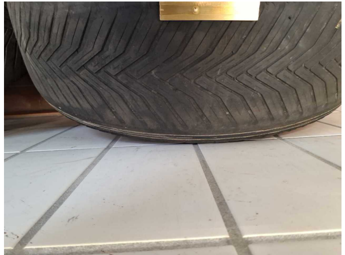
Damage 4: 2nd wheel set: 2 tyres (Sommerreifen) - Worn - Replace
