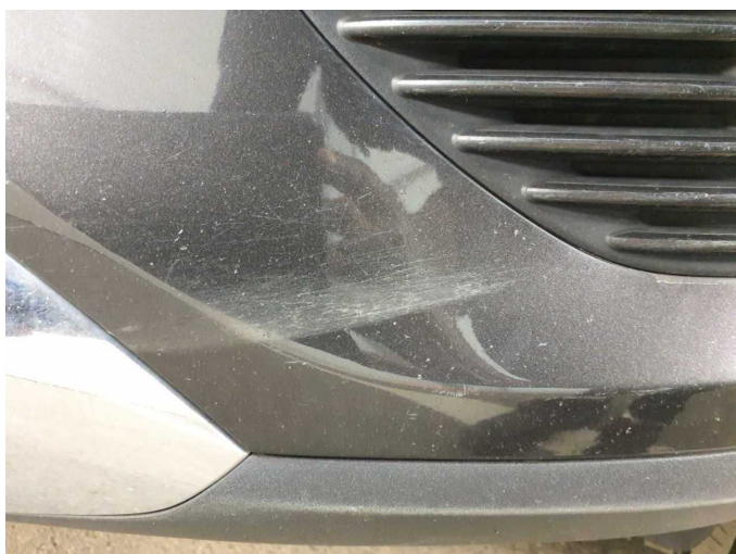
Damage 5: Front bumper: Front bumper - Scratch(es) - Paint
