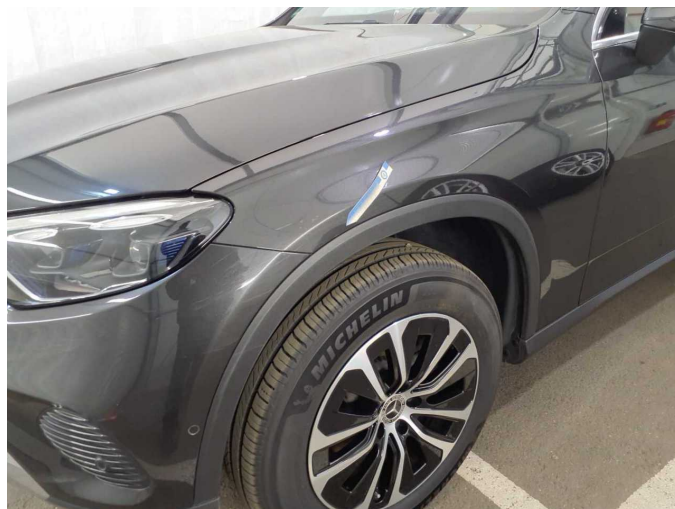
Damage 2: Mudguard - left side: Wheel well extension - Scratch(es) - Loss in value
