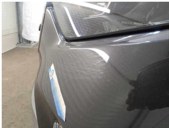
Damage 5: Front bumper: Front bumper - Scratch(es) - Paint
