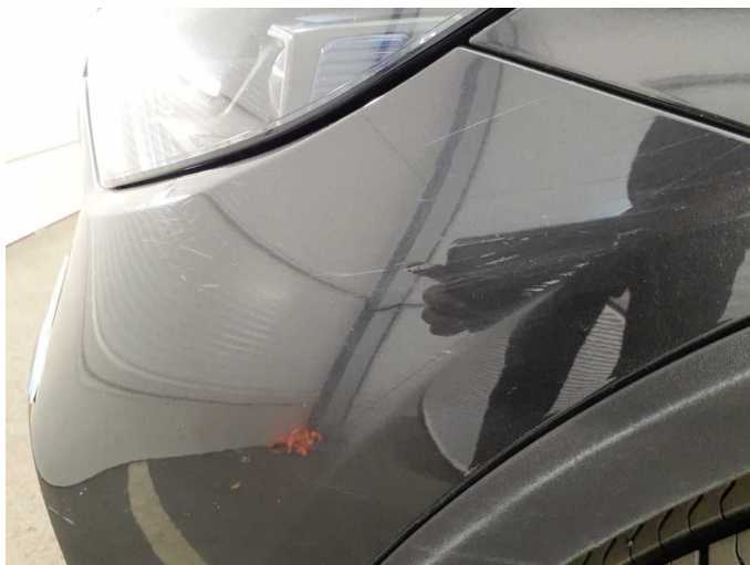
Damage 5: Front bumper: Front bumper - Scratch(es) - Paint
