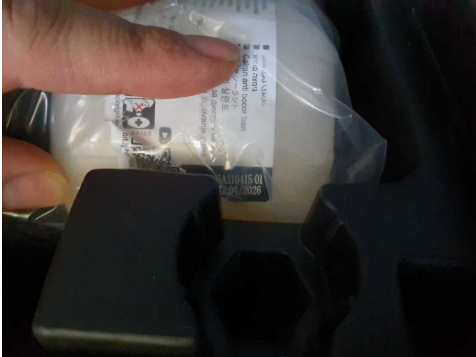
Damage 1: Equipment: Tirefit filler - Expired - Replace
