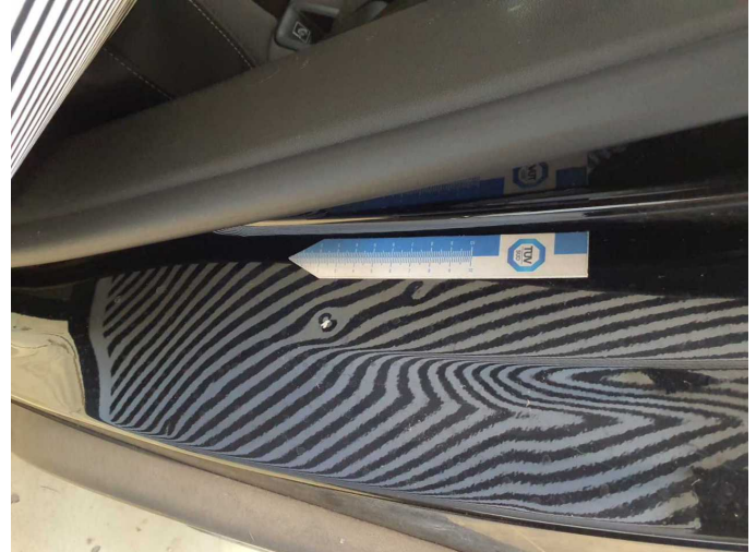
Damage 10: Side panel - rear left side: Sill - Dent / paintcoat damage - Smart repair
