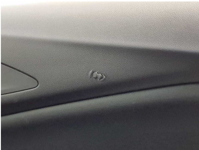
Damage 16: Trim / covers: Door trim - front right side - Scratched - Replace
