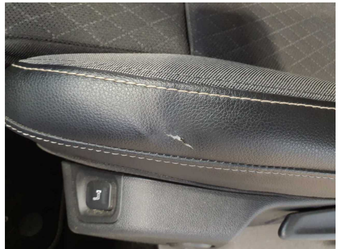
Damage 8: Seat - front: Seat cover - left side - Scratch(es) - Smart repair
