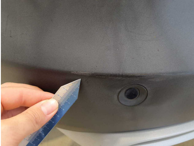
Damage 4: Rear bumper: Spoiler - Scratch(es) - Loss in value
