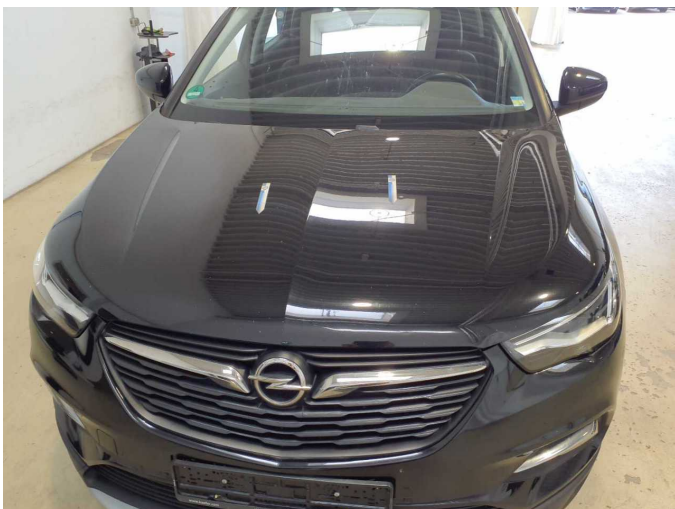
Damage 17: Body: Body - Damage by hail - Smooth repair work
