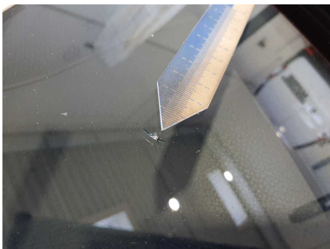
Damage 8: Vehicle glazing: Windscreen - Broken / torn - Replace
