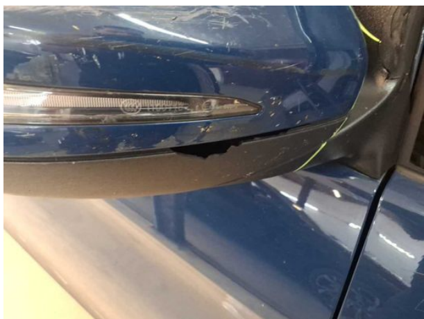
Damage #12: Wing mirror - right side: Mirror housing - Damaged - Replace
