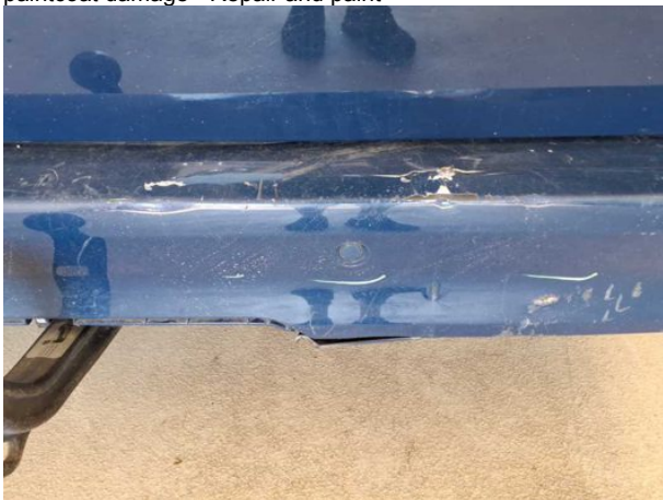
Damage #20: Rear bumper: Rear bumper - Damaged - Replace
