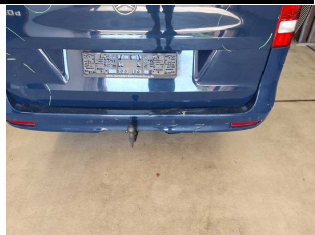
Damage #20: Rear bumper: Rear bumper - Damaged - Replace
