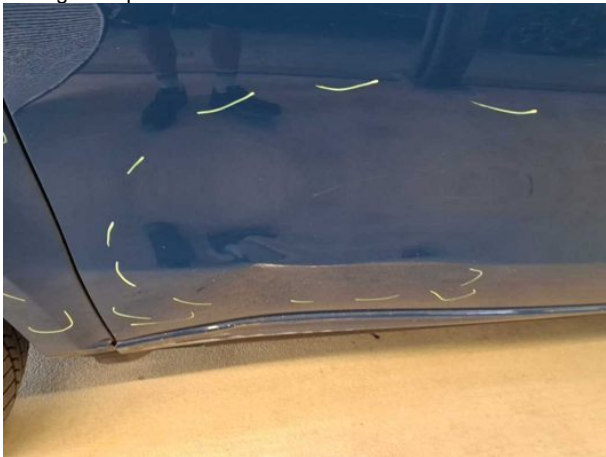
Damage #23: Sliding door, right: Sliding door with glass panel - Dent / paintcoat damage - Replace
