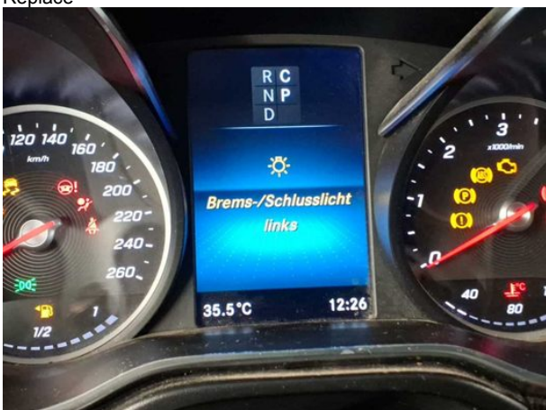
Damage #5: Electrical system: Lighting system - Replace
