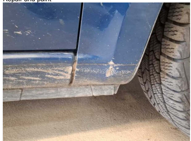
Damage #14: Sill - right side: Sill - Dent / paintcoat damage - Repair and paint
