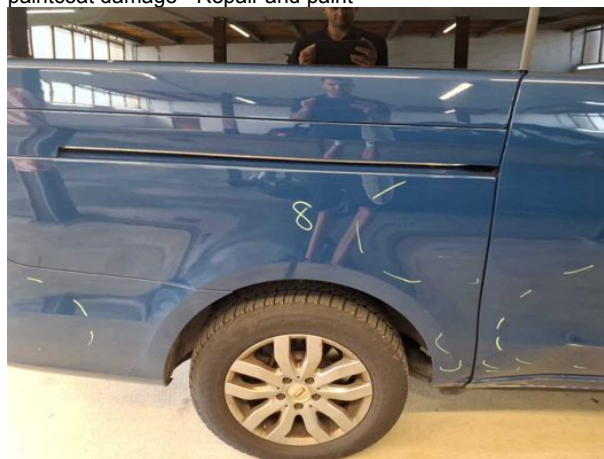
Damage #19: Side panel - rear right side: Side panel - Dent / paintcoat damage - Repair and paint
