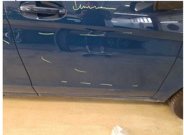
Damage #17: Door - front right side: Door - Scratched - Repair and paint
