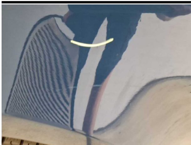
Damage #18: Side panel - rear left side: Side panel - Dent / paintcoat damage - Repair and paint
