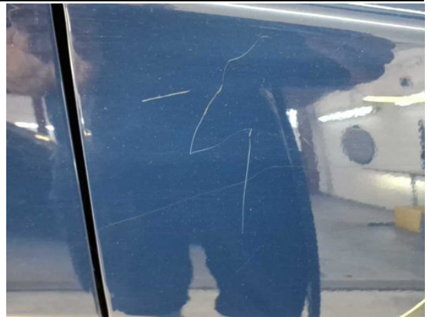
Damage #13: Mudguard - right side: Mudguard - right side - Scratched - Repair and paint
