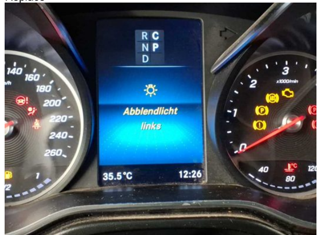
Damage #5: Electrical system: Lighting system - Replace
