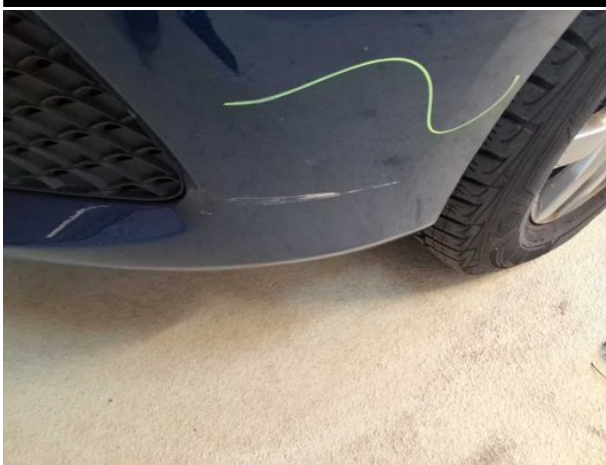
Damage #21: Front bumper: Front bumper - Damaged - Replace
