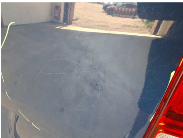
Damage #22: Boot lid / rear door: Boot lid - Dent / paintcoat damage - Replace
