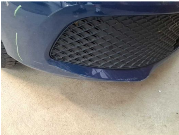
Damage #21: Front bumper: Front bumper - Damaged - Replace
