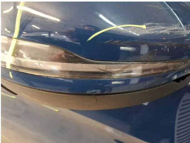
Damage #4: Indicator - front: Mirror - right side - Damaged - Replace
