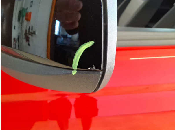
Damage #1: Wing mirror - left side: Cap - Scratched - Smart repair
