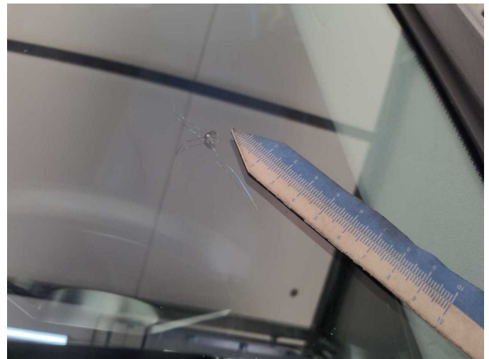
Damage 2: Vehicle glazing: Windscreen with lane departure assistant - Broken / torn - Replace
