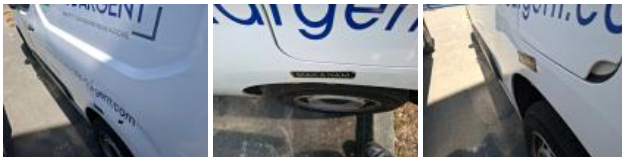
Door FL, Dent(s), Repair and paint (complete)
