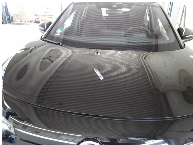
Damage 2: Bonnet: Bonnet - dent(s) - Smart repair
