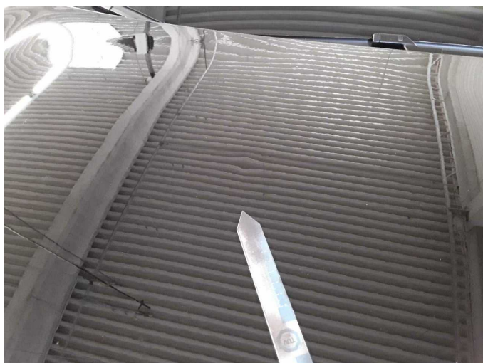
Damage 2: Bonnet: Bonnet - dent(s) - Smart repair
