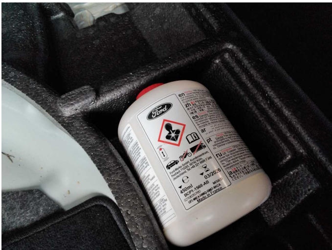
Damage 1: Equipment: Tirefit filler - Expired - Replace
