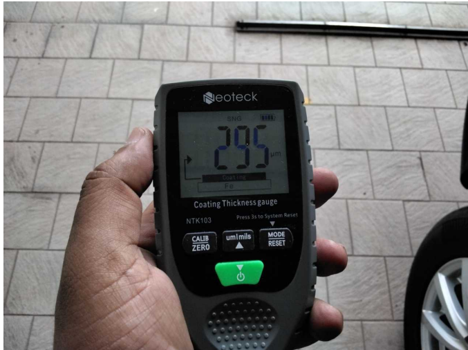
Side panel - rear right side: 295 µm
