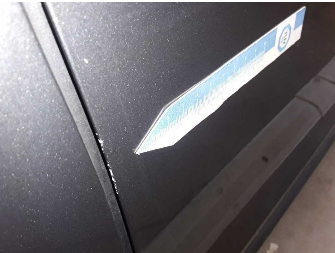
Damage 1: Door - front right side: Door - Scratch(es) - Smart repair
