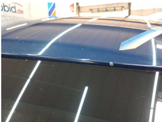
Damage 4: Roof: Roof - Stone chips - Smart repair
