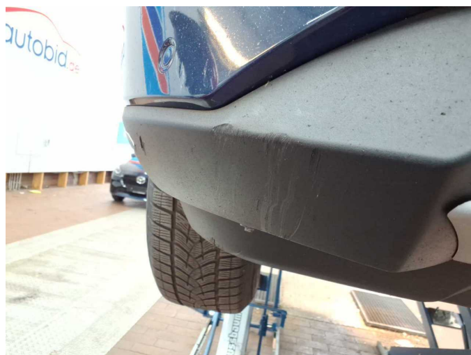
Damage 5: Front bumper: Spoiler - Scratch(es) - Replace
