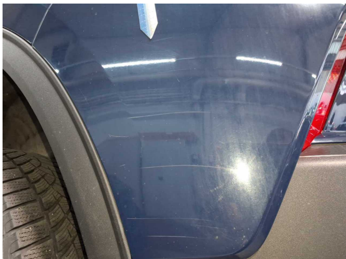
Damage 6: Rear bumper: Rear bumper - Scratch(es) - Paint
