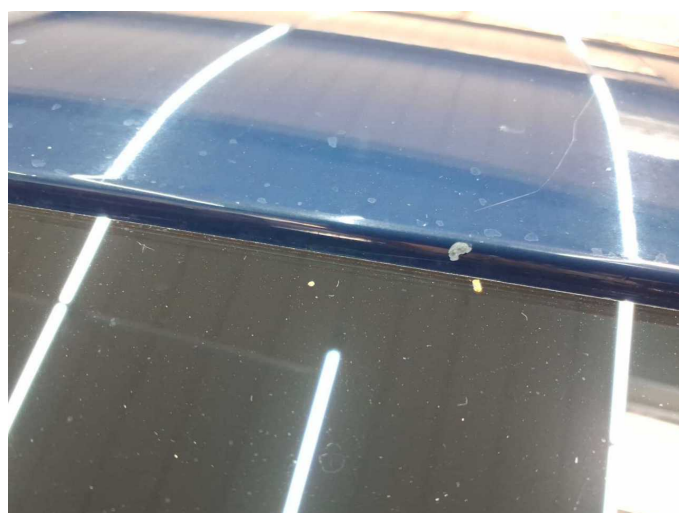
Damage 4: Roof: Roof - Stone chips - Smart repair
