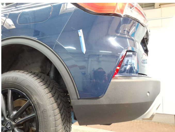
Damage 6: Rear bumper: Rear bumper - Scratch(es) - Paint
