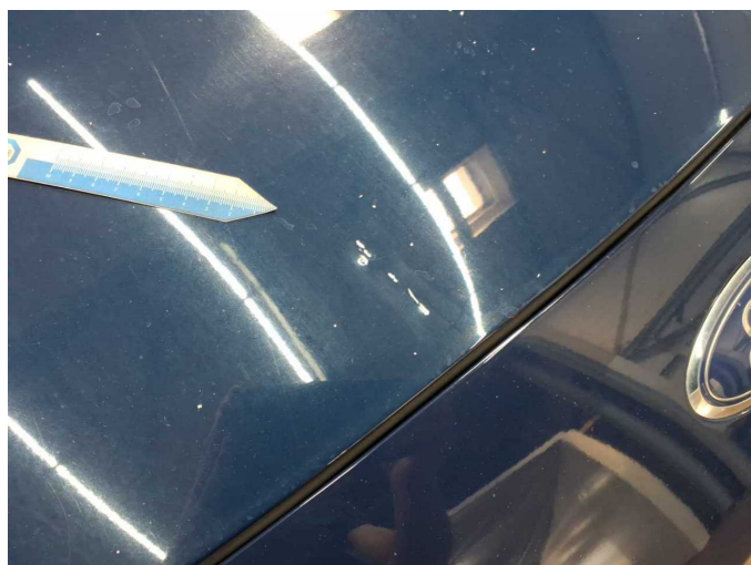
Damage 7: Bonnet: Bonnet (+Steinschläge) - Dent / paintcoat damage - Repair and paint
