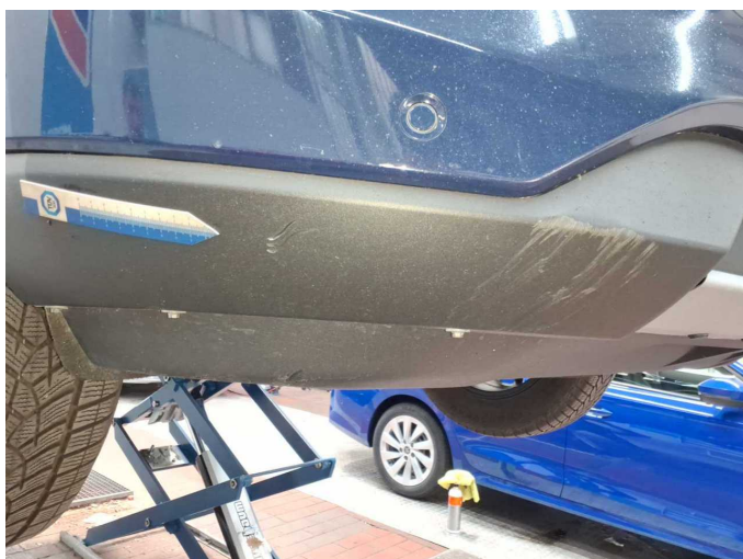
Damage 5: Front bumper: Spoiler - Scratch(es) - Replace
