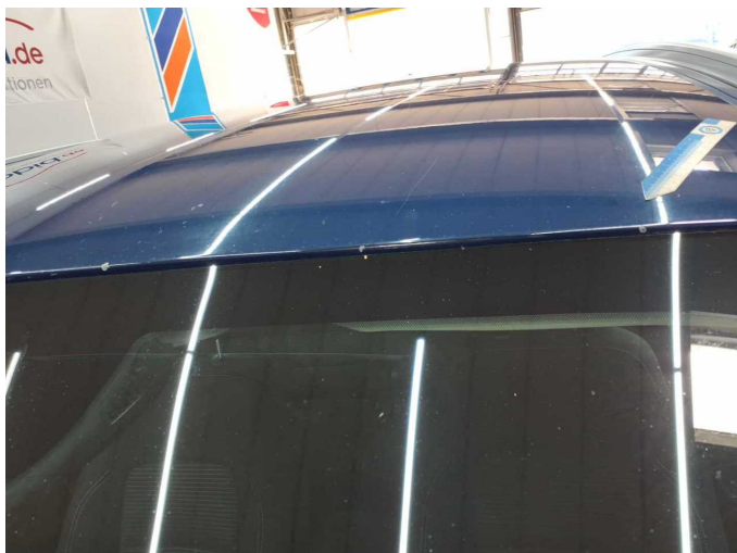
Damage 4: Roof: Roof - Stone chips - Smart repair
