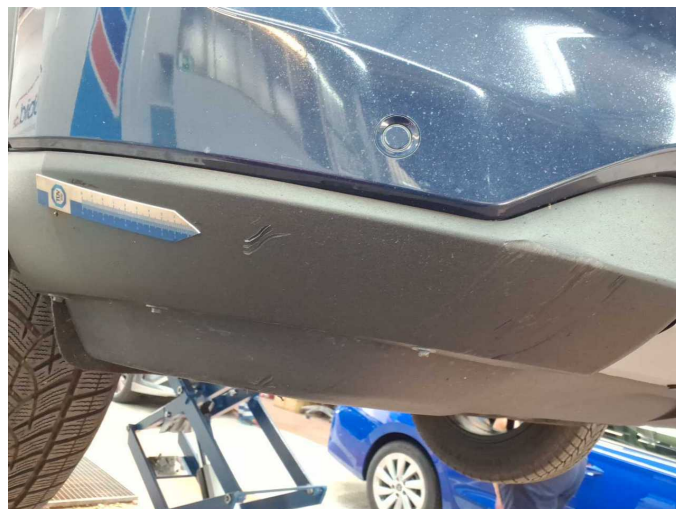
Damage 5: Front bumper: Spoiler - Scratch(es) - Replace
