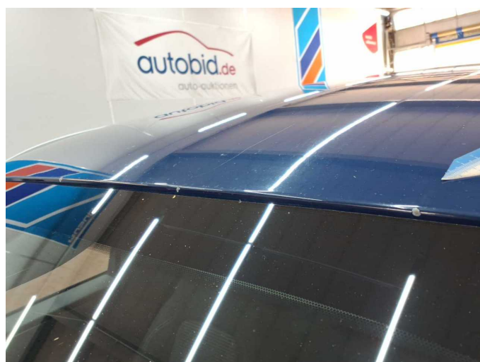
Damage 4: Roof: Roof - Stone chips - Smart repair
