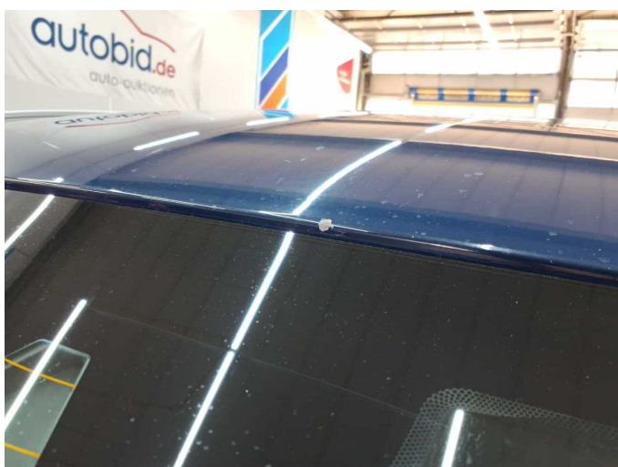
Damage 4: Roof: Roof - Stone chips - Smart repair
