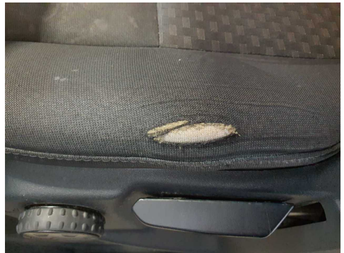
Damage 5: Seat - front: Seat upholstery - left side - Broken / torn - Smart repair
