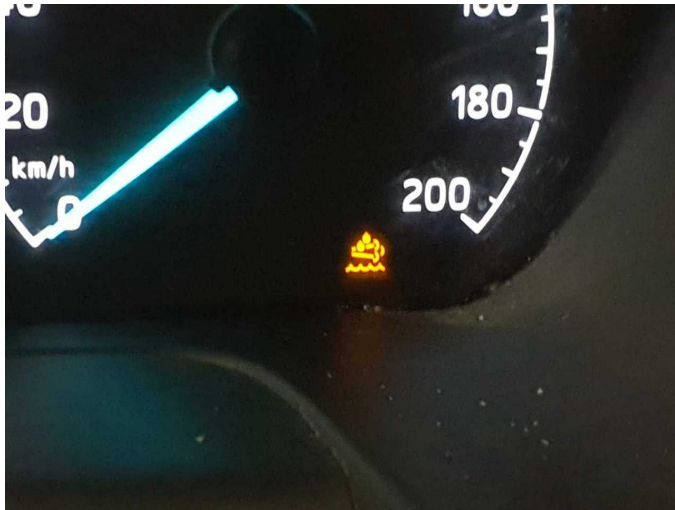
Damage 8: Instrument panel: Indicator light (Abgassystem) - on - Perform diagnosis
