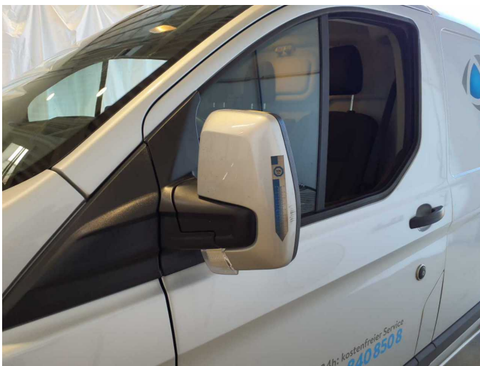
Damage 2: Wing mirror - left side: Cap - Scratch(es) - Paint
