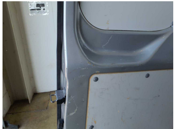
Damage 11: Boot lid / rear door: Rear door - left side - Dent / paintcoat damage - Repair and paint
