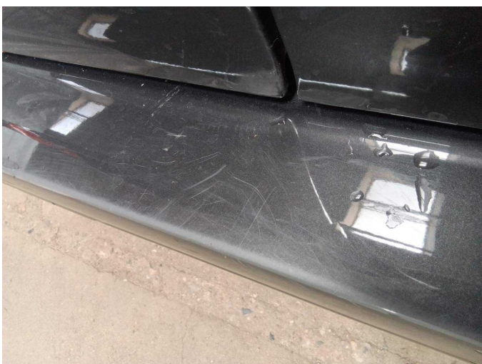
Damage 5: Rear bumper: Rear bumper - Scratch(es) - Paint
