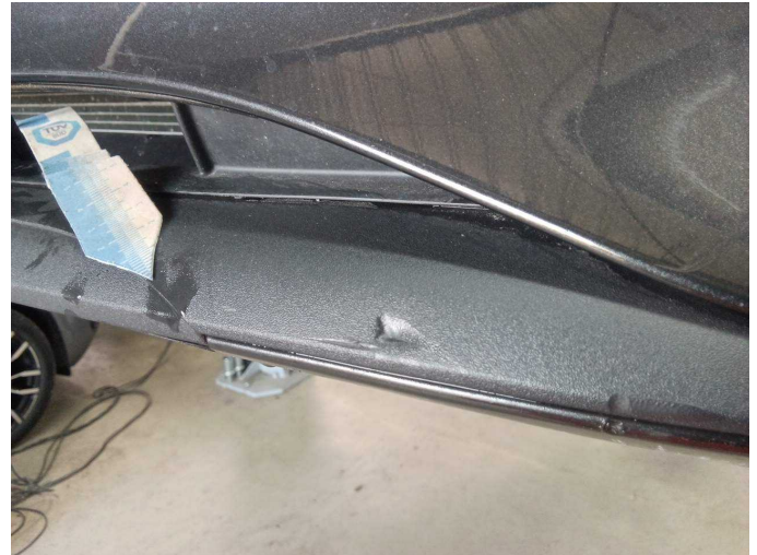
Damage 4: Front bumper: Protection strip - centre - Damaged - Replace
