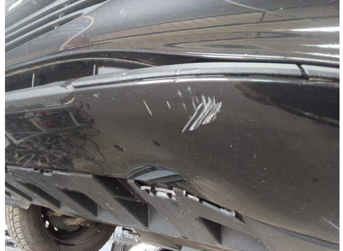
Damage 6: Front bumper: Front bumper - Scratch(es) - Paint
