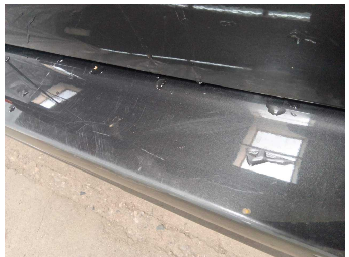
Damage 5: Rear bumper: Rear bumper - Scratch(es) - Paint
