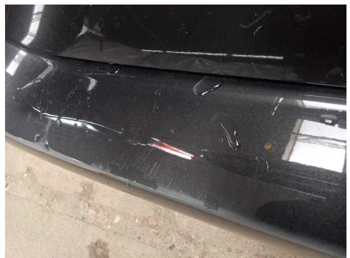
Damage 5: Rear bumper: Rear bumper - Scratch(es) - Paint
