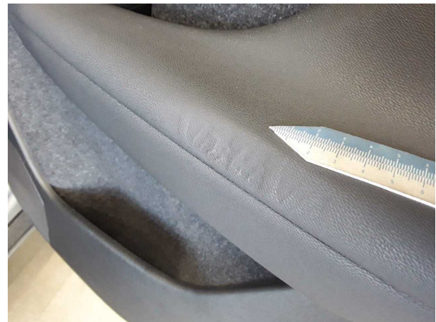
Damage #3: Trim / covers: Door trim - rear right side - Deformed - Replace
