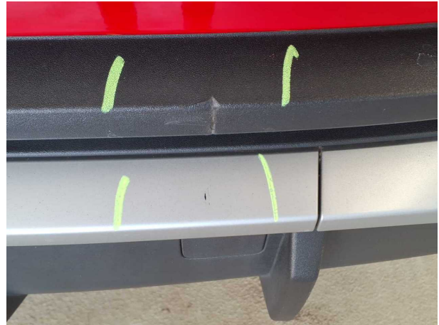
Damage #2: Rear bumper: Spoiler - Deformed - Replace
