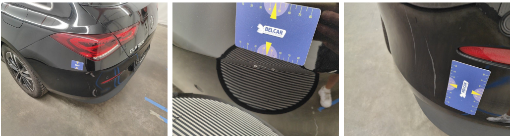
Bumper Rear // Repair & Painting-scratch + dent
