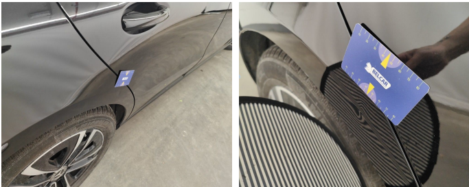
Wing Rear Right // Repair & Painting-dent
