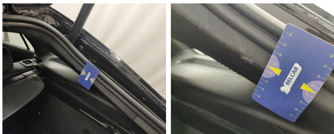
Trunk Compartment / Side Cover Right / Replace-tear
