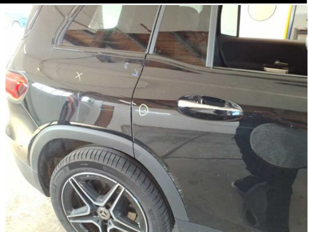
Damage #7: Door - rear right side: Door - Dent / paintcoat damage - Smooth repair work
