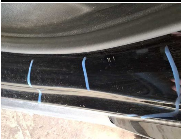
Damage #5: Side panel - rear left side: Sill - Scratch(es) - Cover / polish
