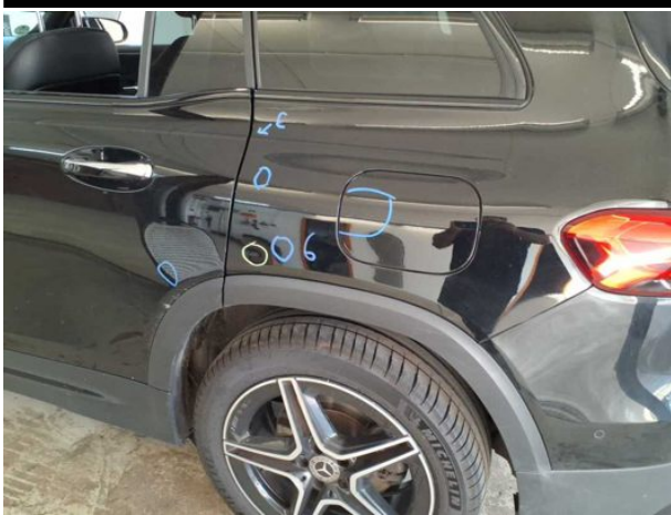
Damage #15: Side panel - rear left side: Side panel - Dent / paintcoat damage - Repair and paint
