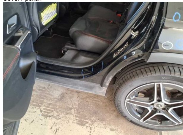
Damage #5: Side panel - rear left side: Sill - Scratch(es) - Cover / polish
