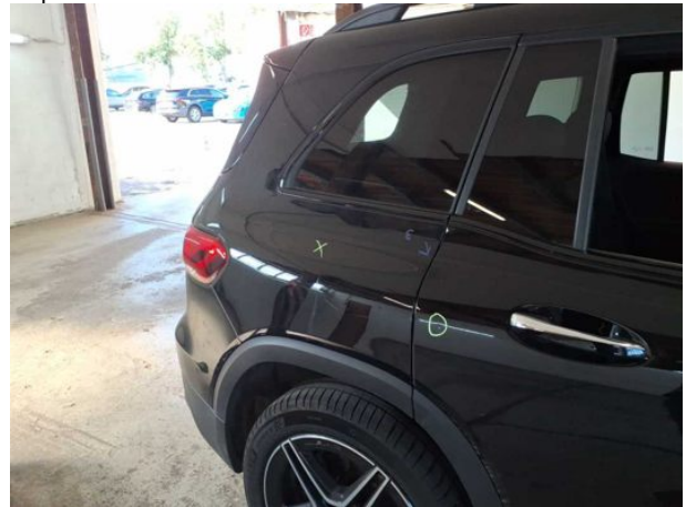
Damage #14: Side panel - rear right side: Side panel - Unprofessionally repaired - Repair and paint
