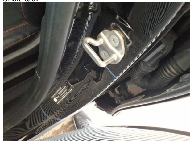
Damage #10: Sill - left side: Sill - Dent / paintcoat damage - Smart repair
