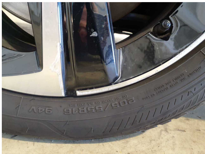
Damage 9: Wheel / tyres: Alloy rim - front left side - Scratch(es) - Replace
