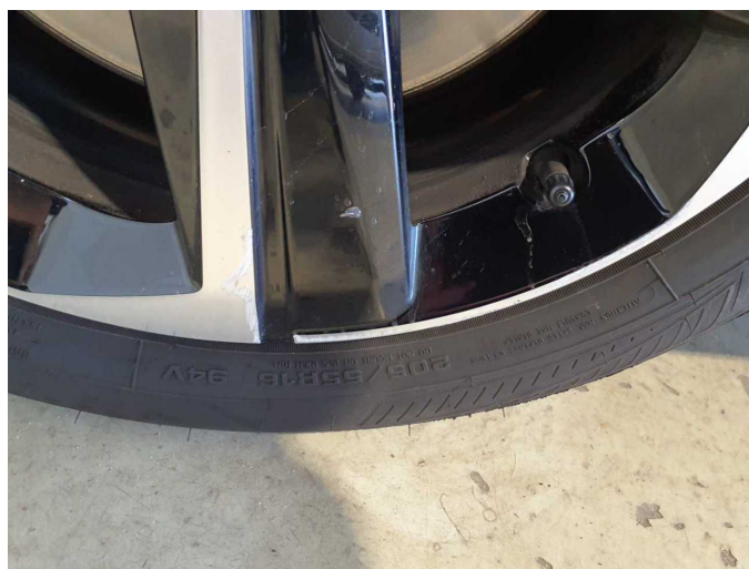
Damage 9: Wheel / tyres: Alloy rim - front left side - Scratch(es) - Replace
