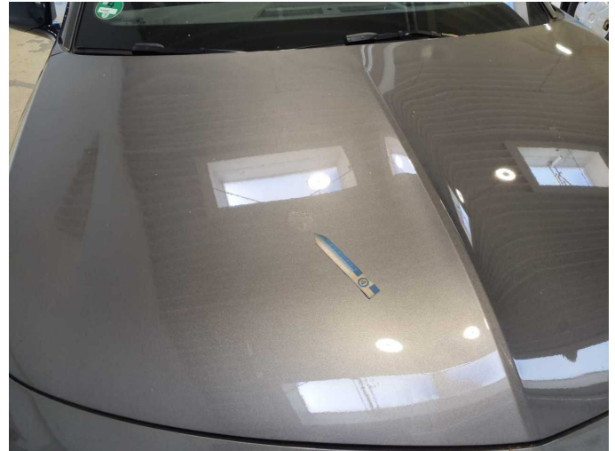
Damage 13: Bonnet: Bonnet (Anätzung) - Paint defect - Repair and paint
