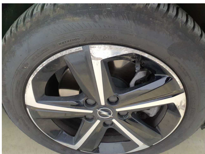
Damage 10: Wheel / tyres: Alloy rim - front right side - Scratch(es) - Replace
