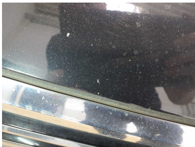
Damage 19: Bonnet: Bonnet - Corrosion - Repair and paint
