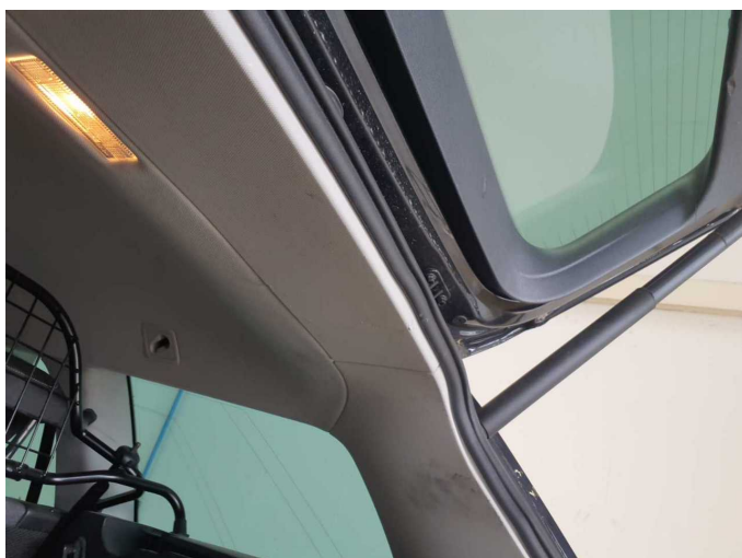
Damage 6: Trim / covers: Boot lining - Scratch(es) - Replace
