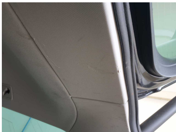
Damage 6: Trim / covers: Boot lining - Scratch(es) - Replace
