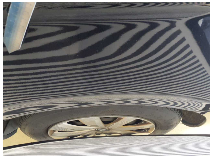
Damage 14: Side panel - rear left side: Side panel (Spachtel eingefallen) - Unprofessionally repaired - Repair and paint
