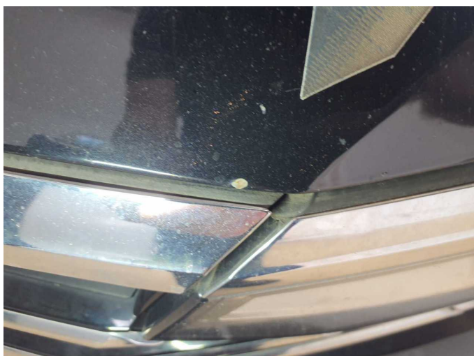
Damage 19: Bonnet: Bonnet - Corrosion - Repair and paint
