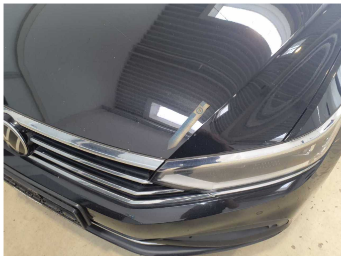
Damage 19: Bonnet: Bonnet - Corrosion - Repair and paint
