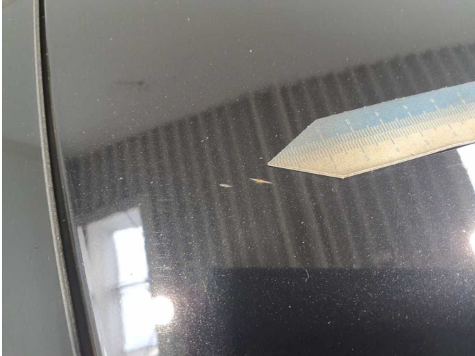
Damage 20: Roof: Roof - Corrosion - Repair and paint
