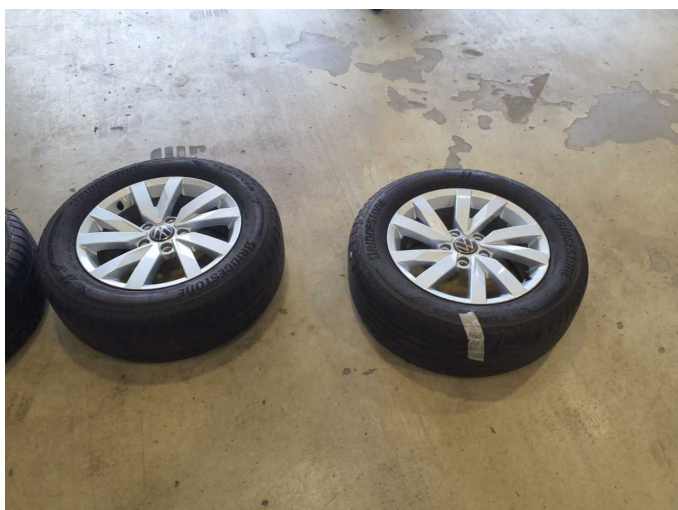
Damage 9: 2nd wheel set: 2 tyres - Worn - Replace
