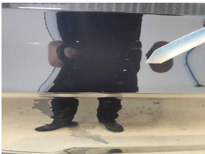
Damage 16: Door - rear right side: Door - Dent / paintcoat damage - Repair and paint
