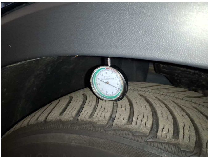
Damage 1: Wheel / tyres: Tyre - front left side - Does not meet the leasing specifications - Replace
