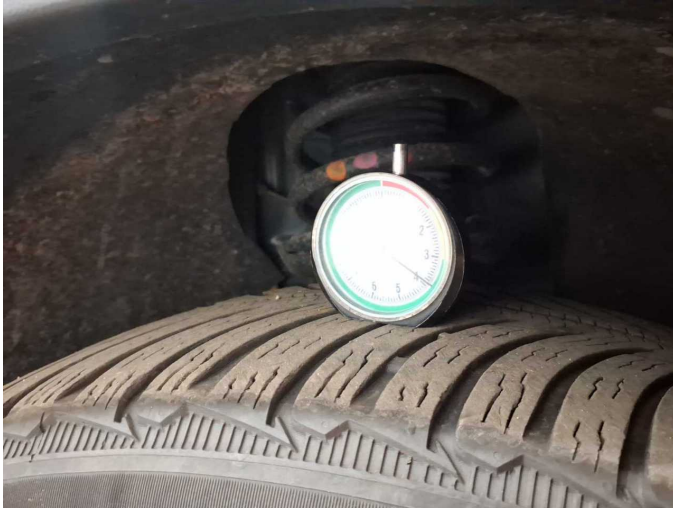
Damage 2: Wheel / tyres: Tyre - front right side - Does not meet the leasing specifications - Replace
