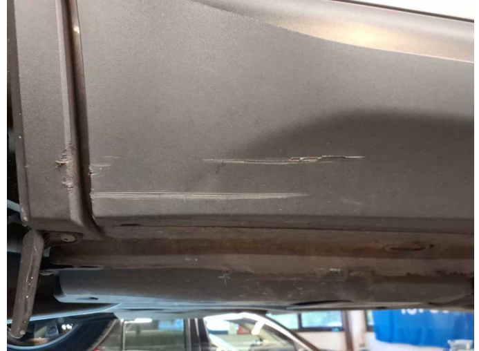
Damage 3: Door - rear right side: Brightware - lower - Scratch(es) - Replace
