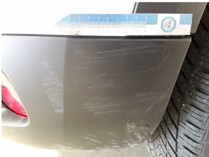
Damage 5: Rear bumper: Spoiler - Scratch(es) - Replace
