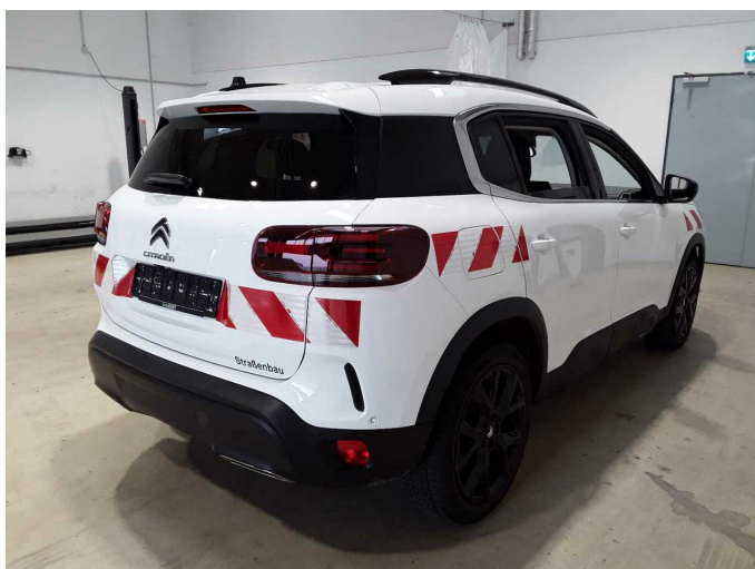
Damage 3: Body: Body - Glued / labelled - De-glue / neutralise
