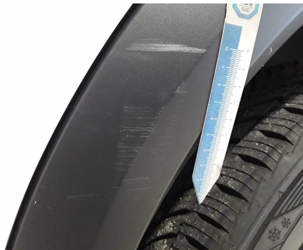
Damage 1: Side panel - rear left side: Wheel well extension - Scratch(es) - Replace
