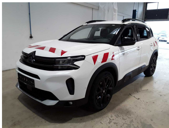
Damage 3: Body: Body - Glued / labelled - De-glue / neutralise
