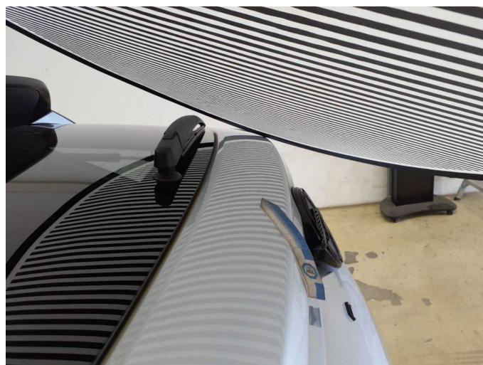
Wear and tear 7: Boot lid / rear door: Boot lid - dent(s) - No deduction
