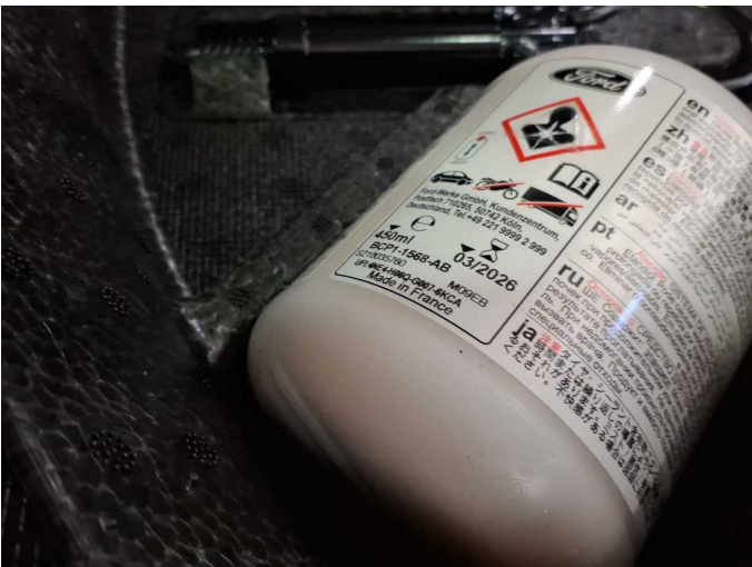
Damage 1: Equipment: Tirefit filler - Due - Replace
