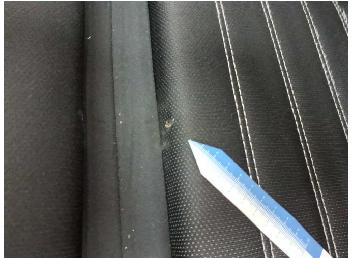
Damage 7: Seat - front: Seat cover - left side - Burn hole (cigarettes) - Smart repair
