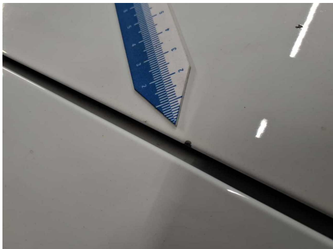
Damage 10: Bonnet: Bonnet - Stone chips - Paint
