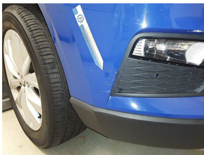
Damage 14: Front bumper: Front bumper - Dent / paintcoat damage - Paint
