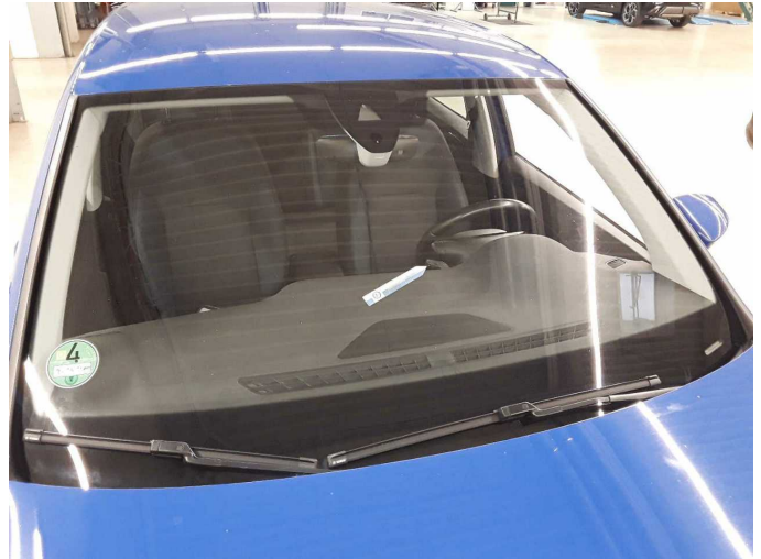
Damage 16: Vehicle glazing: Windscreen - Stone chips - Replace
