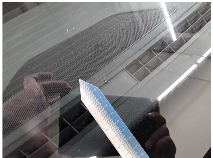
Damage 16: Vehicle glazing: Windscreen - Stone chips - Replace
