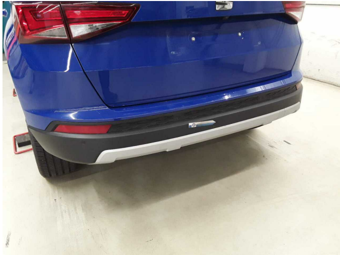
Wear and tear 6: Rear bumper: Spoiler - Scratch(es) - No deduction
