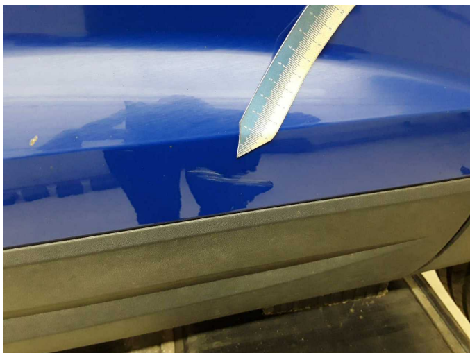
Damage 15: Door - front right side: Door - Dent / paintcoat damage - Paint
