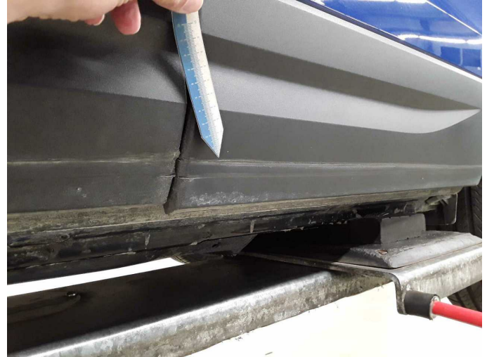
Damage 10: Door - rear left side: Brightware - lower - Scratched - Replace
