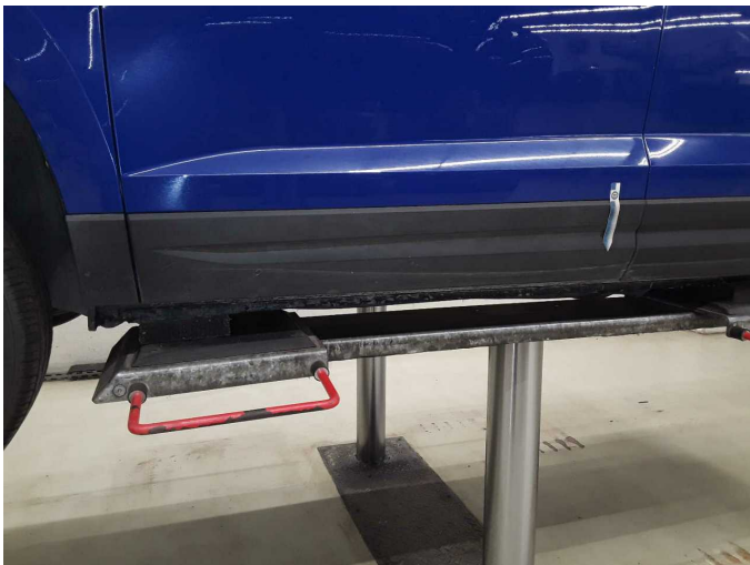
Damage 11: Door - front left side: Brightware - lower - Scratched - Replace
