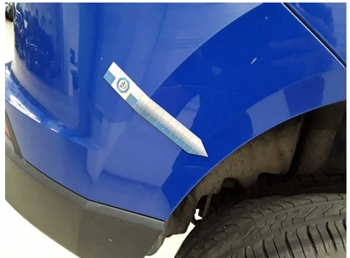
Damage 12: Rear bumper: Rear bumper - Scratch(es) - Paint
