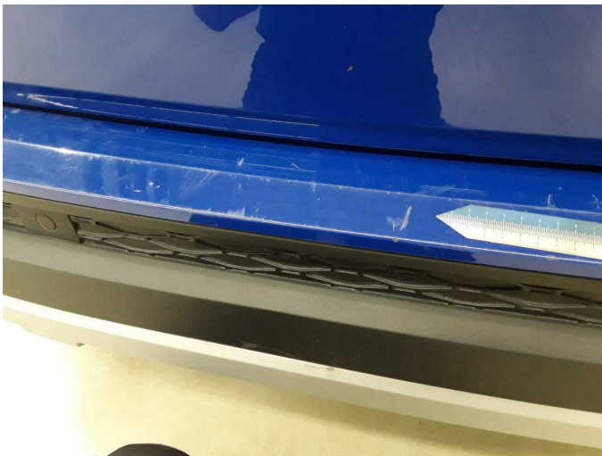
Damage 12: Rear bumper: Rear bumper - Scratch(es) - Paint
