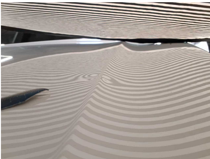
Damage 8: Bonnet: Bonnet - Deformed - Repair and paint
