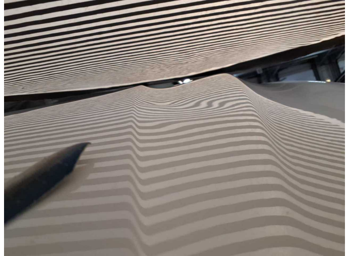
Damage 8: Bonnet: Bonnet - Deformed - Repair and paint
