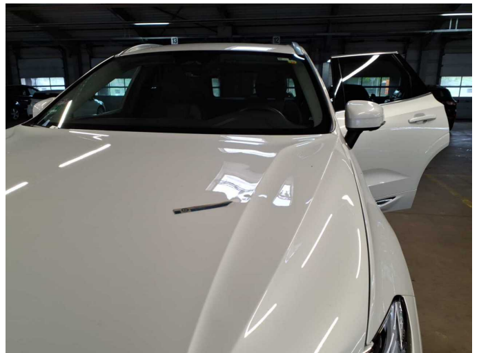
Damage 8: Bonnet: Bonnet - Deformed - Repair and paint
