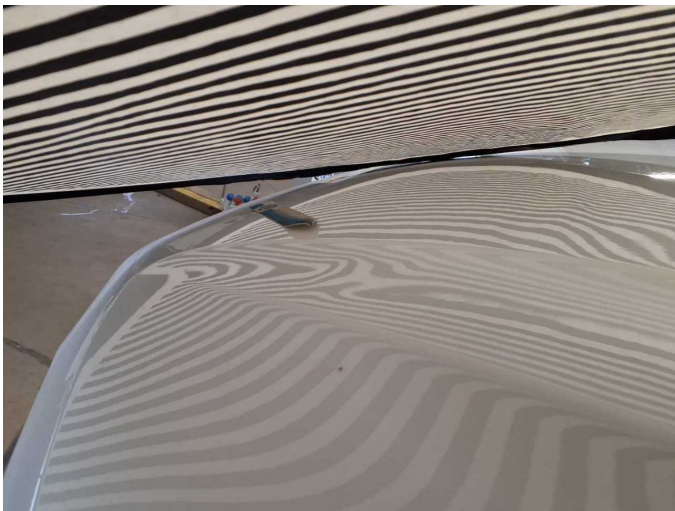
Damage 8: Bonnet: Bonnet - Deformed - Repair and paint
