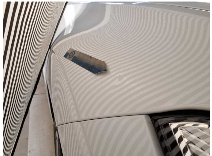
Damage 2: Mudguard - right side: Mudguard - right side - dent(s) - Smooth repair work
