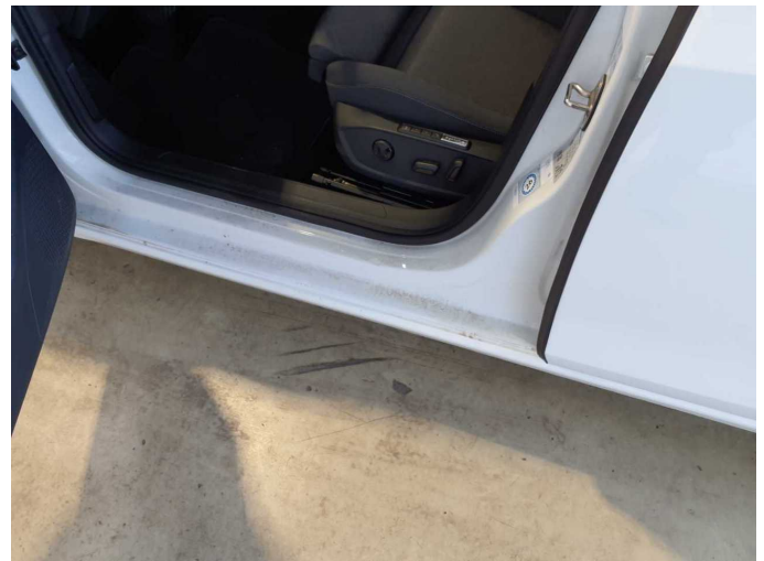
Damage 4: Sill - left side: Sill - Dent / paintcoat damage - Smart repair
