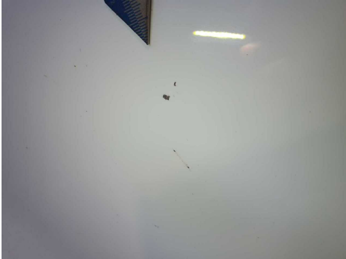
Damage 5: Door - front right side: Door - Scratch(es) - Smart repair
