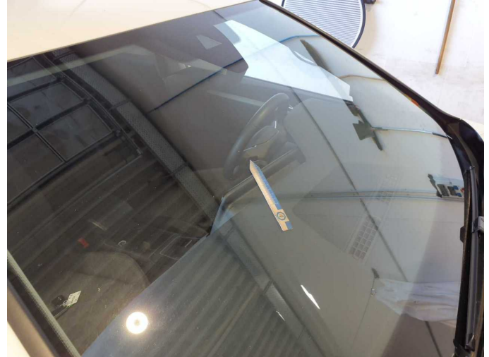
Damage 8: Vehicle glazing: Windscreen (kein Staubschutz) - Stone chips - repair according to calculation
