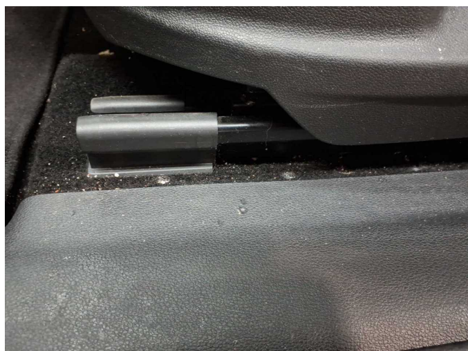
Damage 5: Trim / covers: Carpet (+ Einstiegsleiste links) - Holes - Smart repair
